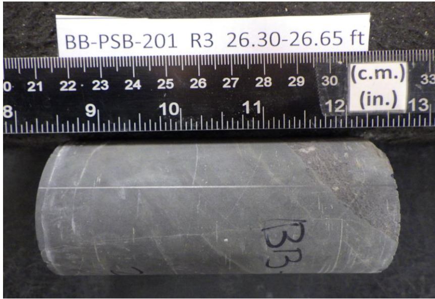
After cutting and grinding
