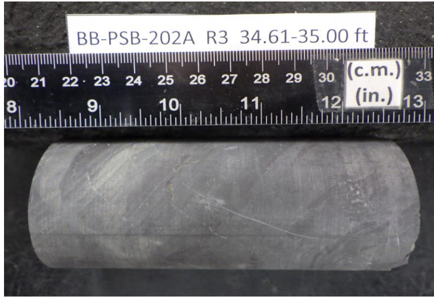
After cutting and grinding
