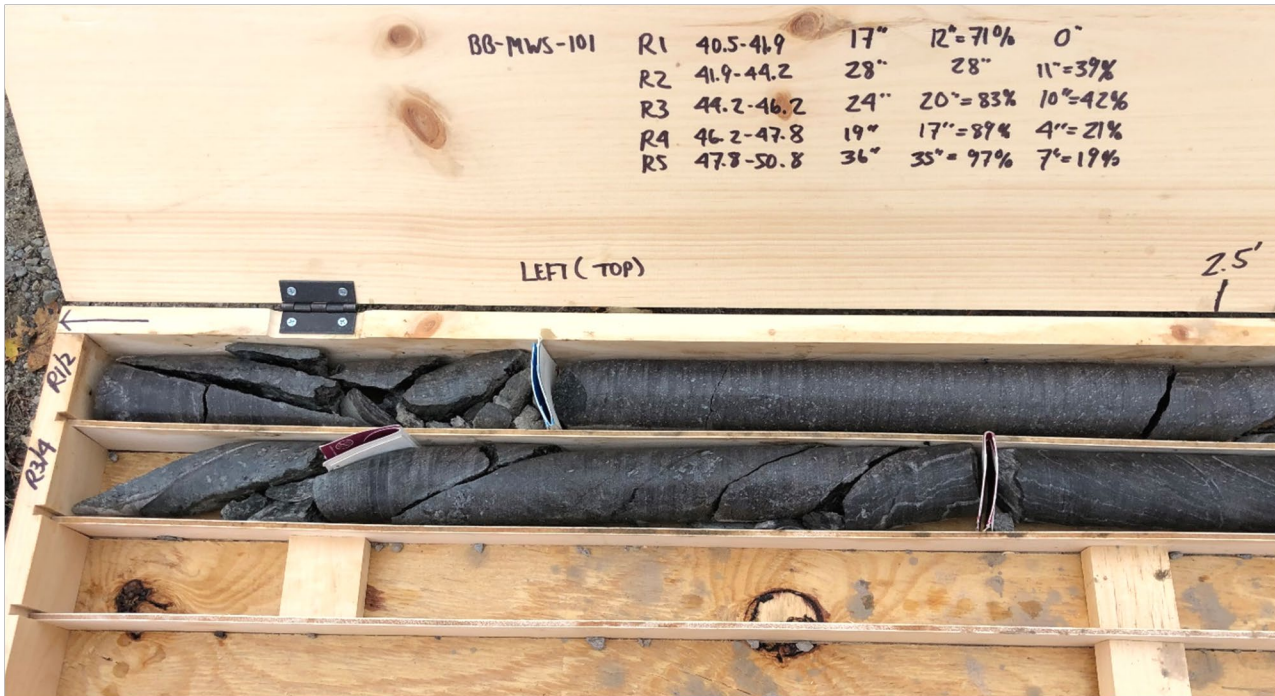
Core box containing wetted core from test boring BB-MWS-101 (Box 1 of 1); left side of core box (top portion of cores). Slots from top to bottom:
