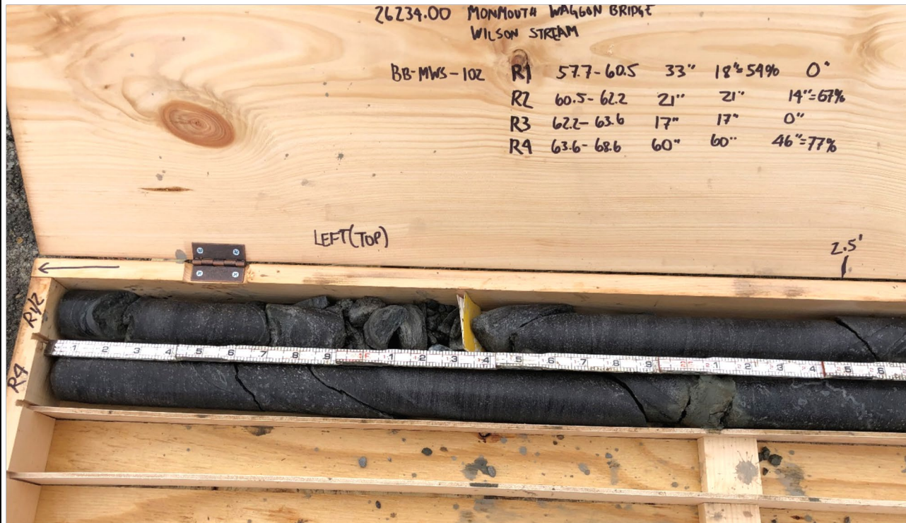
Core box containing wetted core from test boring BB-MWS-102 (Box 1 of 1); left side of core box (top portion of cores). Slots from top to bottom:
