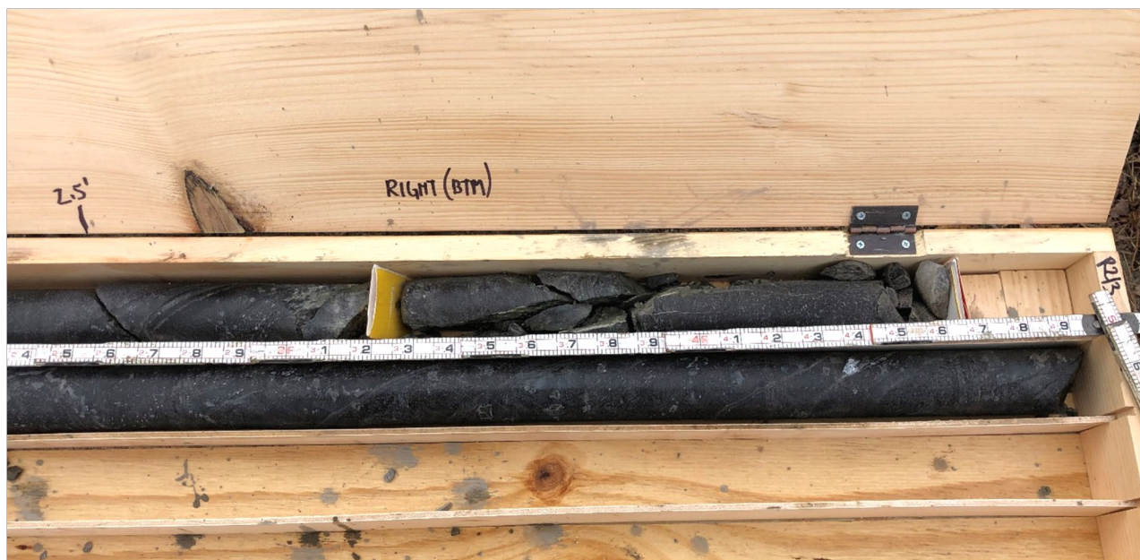
Core box containing wetted core from test boring BB-MWS-102 (Box 1 of 1); right side of core box (bottom portion of cores). Slots from top to bottom:
