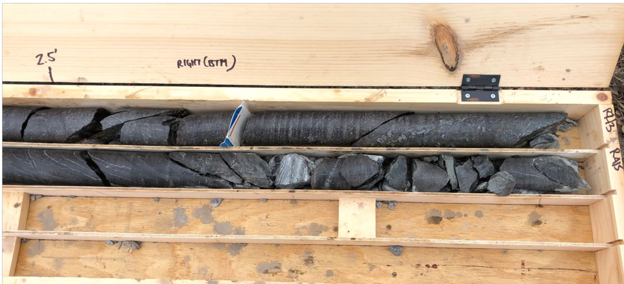
Core box containing wetted core from test boring BB-MWS-101 (Box 1 of 1); right side of core box (bottom portion of cores). Slots from top to bottom:
