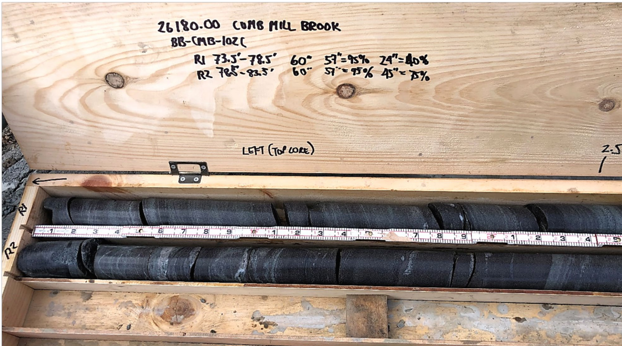
Core box containing wetted core from test boring BB-CMB-102C (Box 1 of 1); left side of core box (top portion of cores). Slots from top to bottom:
