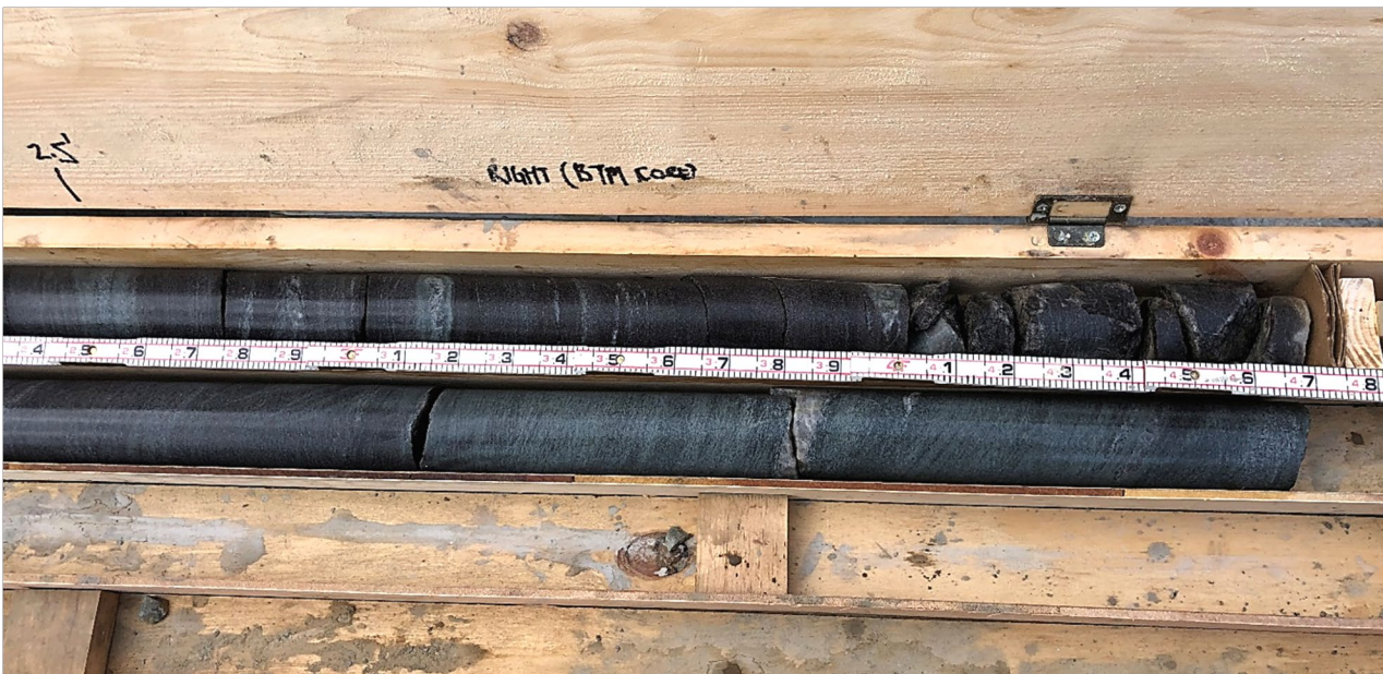
Core box containing wetted core from test boring BB-CMB-102C (Box 1 of 1); right side of core box (bottom portion of cores). Slots from top to bottom:
