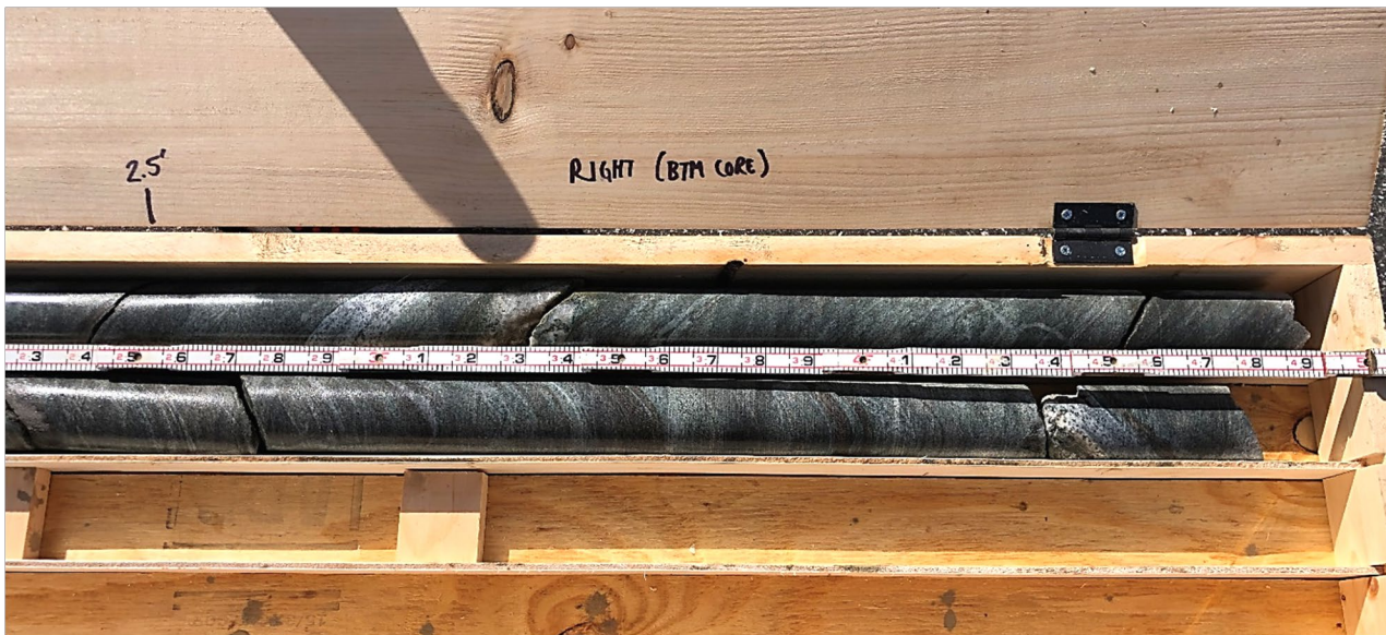
Core box containing wetted core from test boring BB-MMMS-101 (Box 1 of 1); right side of core box (bottom portion of cores). Slots from top to bottom:
