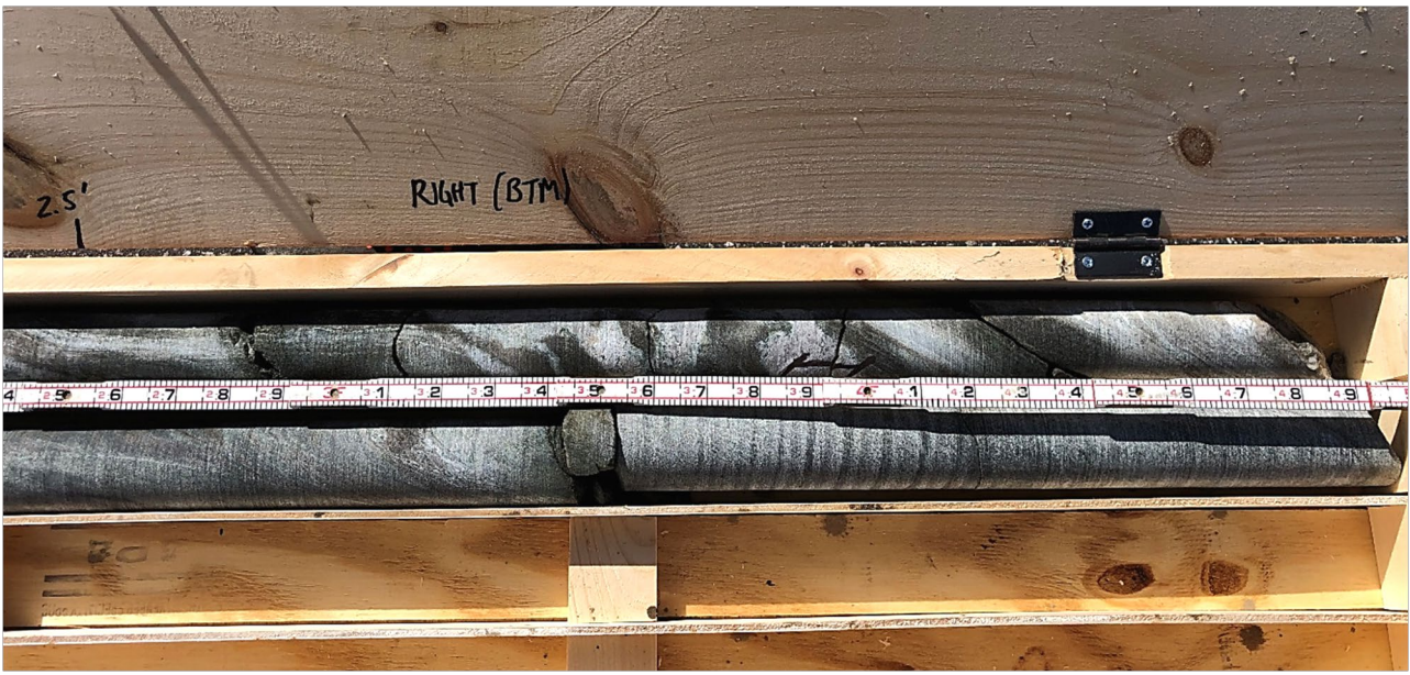
Core box containing wetted core from test boring BB-MMMS-102 (Box 1 of 1); right side of core box (bottom portion of cores). Slots from top to bottom: 1) BB-MMMS-102, R1; 2) BB-MMMS-102, R2; 3) empty; 4) empty.
