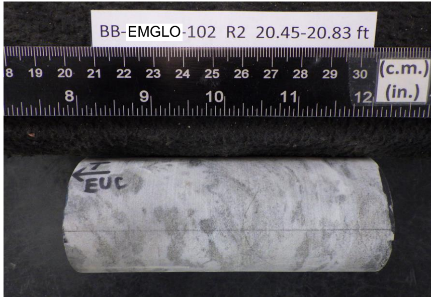
After cutting and grinding
