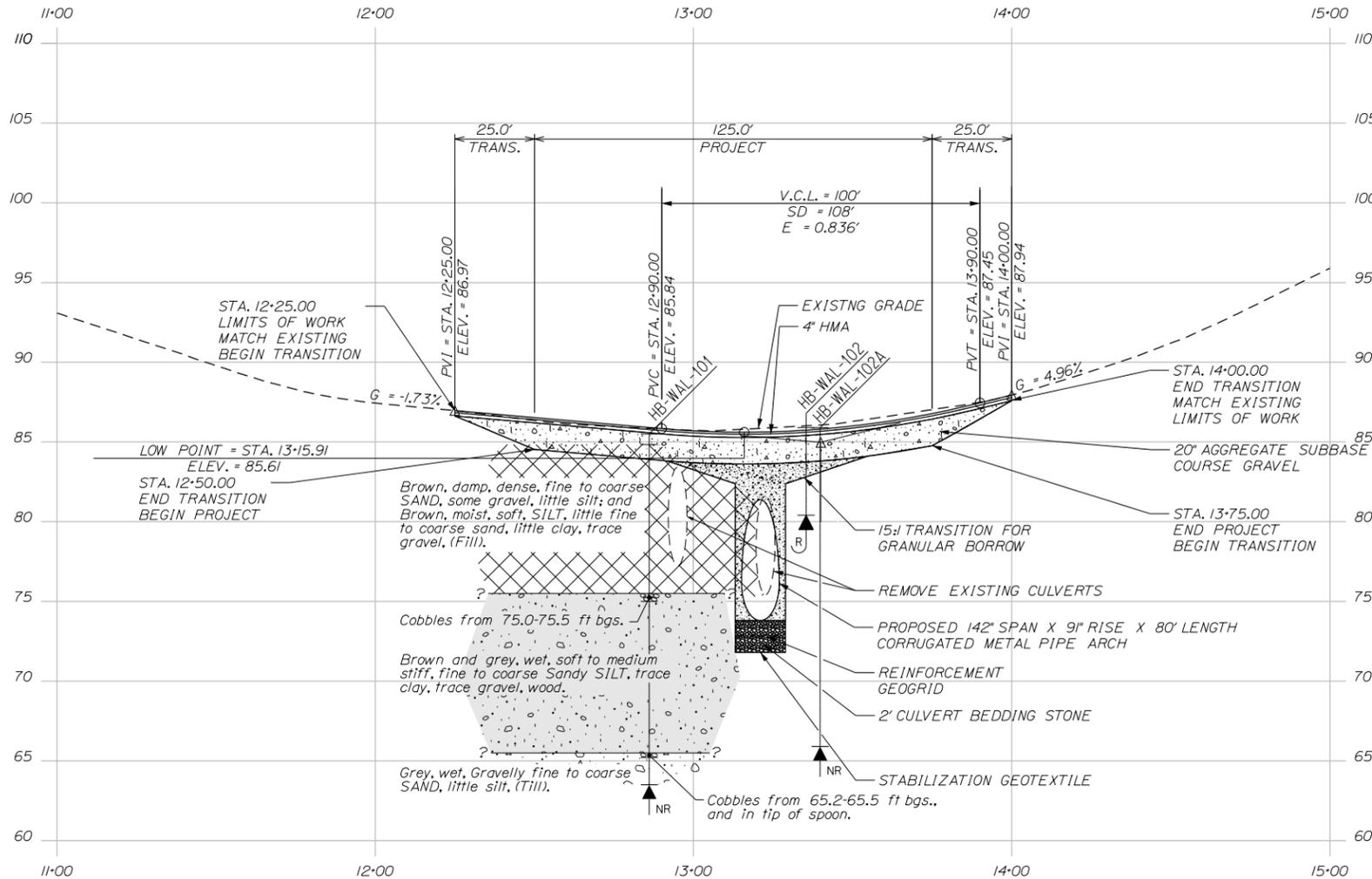
Note: This generalized interpretive soil profile is intended to convey trends in subsurface conditions. The boundaries between strata are approximate and idealized, and have been developed by interpretations of widely spaced explorations and samples. Actual soil and bedrock transitions may vary and are probably more erratic. For more specific information refer to the exploration logs.
