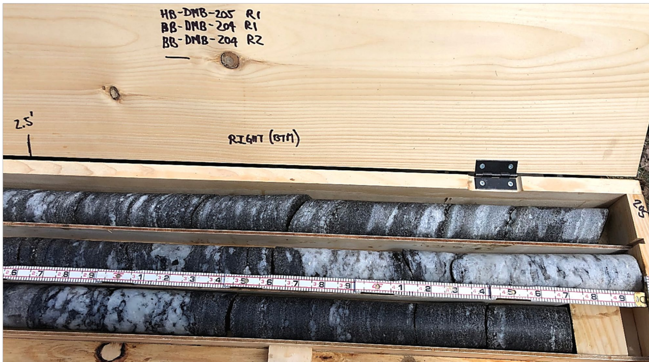
Core box containing wetted core from test borings HB-DMB-205 and BB-DMB-204 (Box 1 of 1); right side of core box (bottom portion of cores). Slots from top to bottom:
