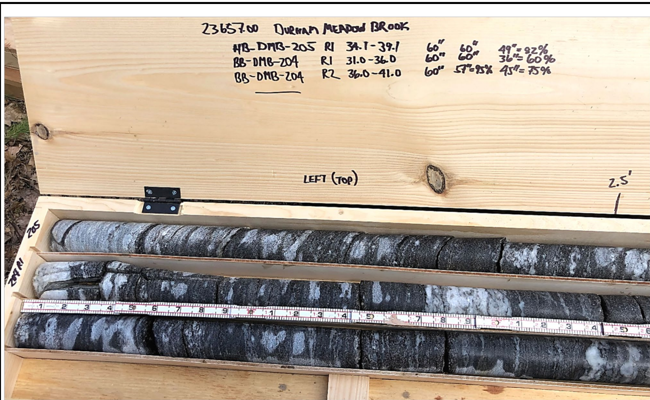
Core box containing wetted core from test borings HB-DMB-205 and BB-DMB-204 (Box 1 of 1); left side of core box (top portion of cores). Slots from top to bottom:
