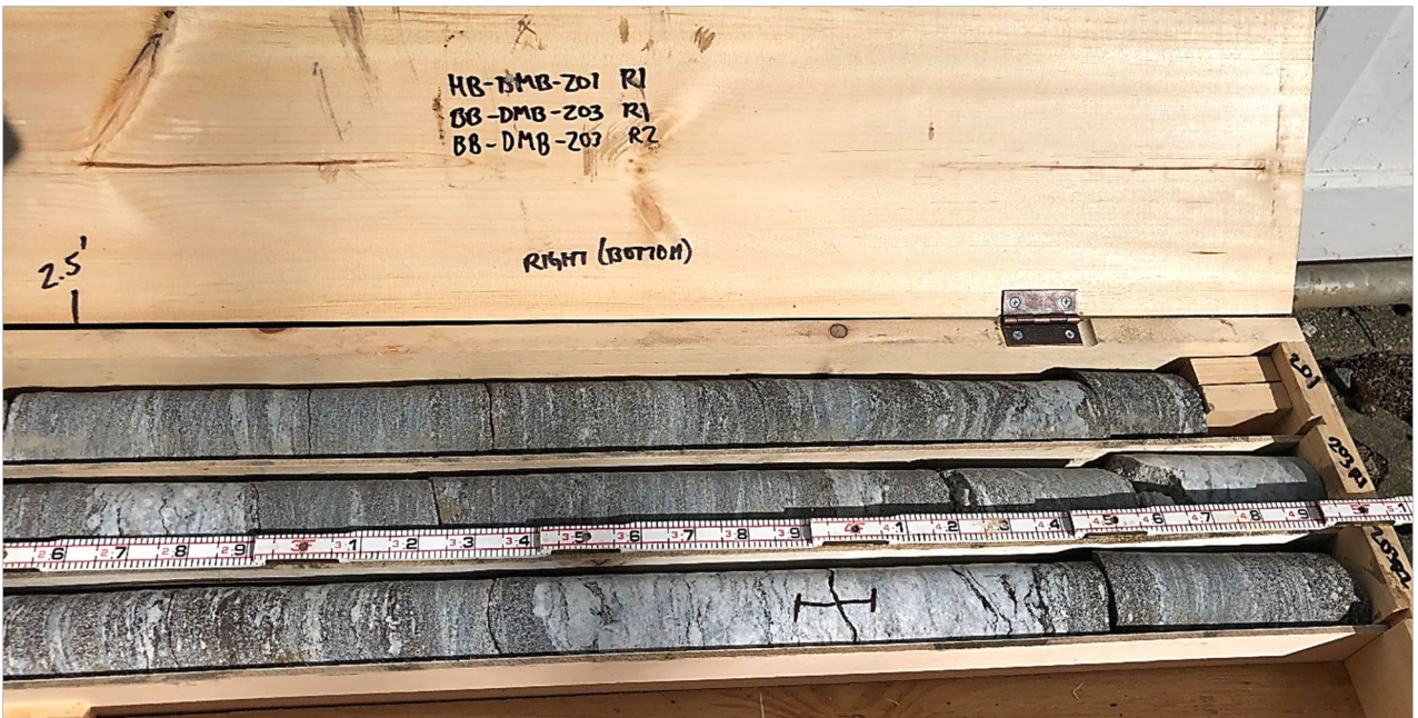
Core box containing dried core from test borings HB-DMB-201 and BB-DMB-203 (Box 1 of 1); right side of core box (bottom portion of cores). Slots from top to bottom:
