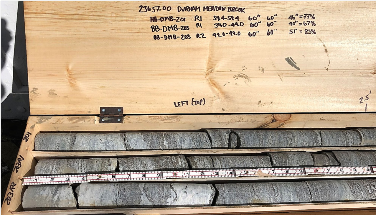
Core box containing dried core from test borings HB-DMB-201 and BB-DMB-203 (Box 1 of 1); left side of core box (top portion of cores). Slots from top to bottom:
