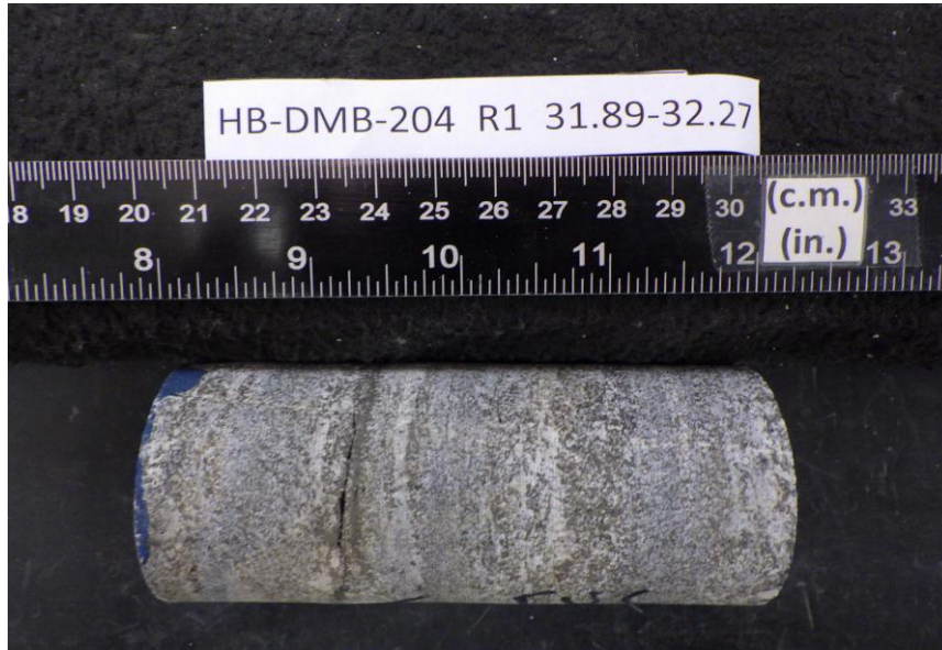
After cutting and grinding
