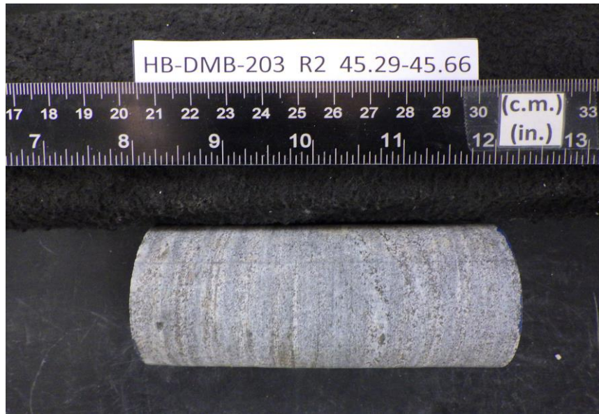
After cutting and grinding
