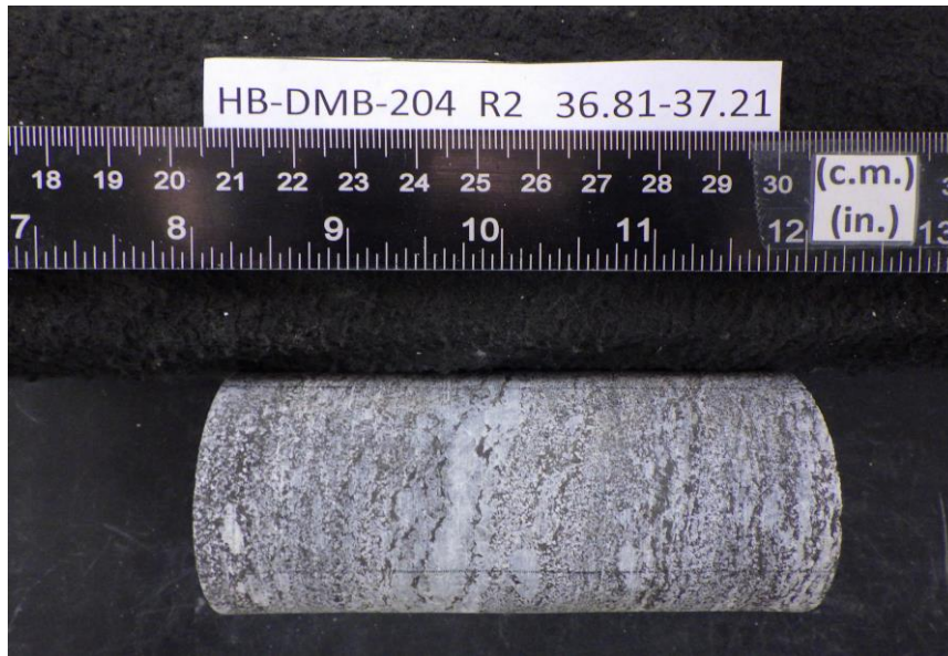
After cutting and grinding
