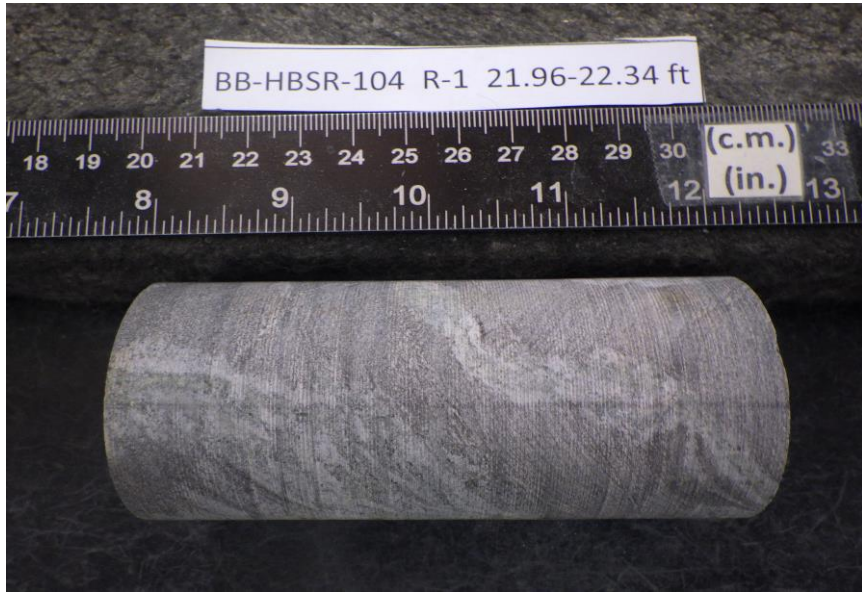
After cutting and grinding
