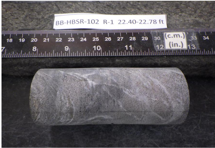
After cutting and grinding
