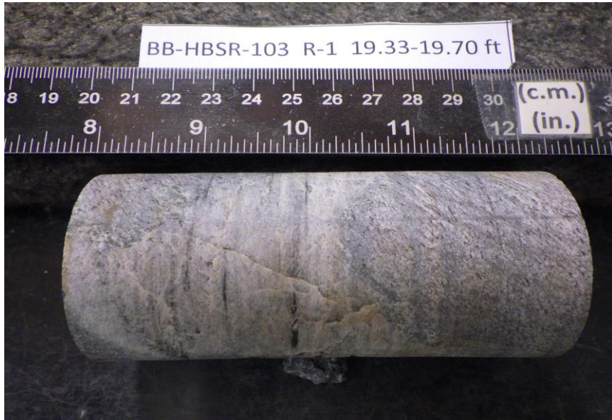
After cutting and grinding
