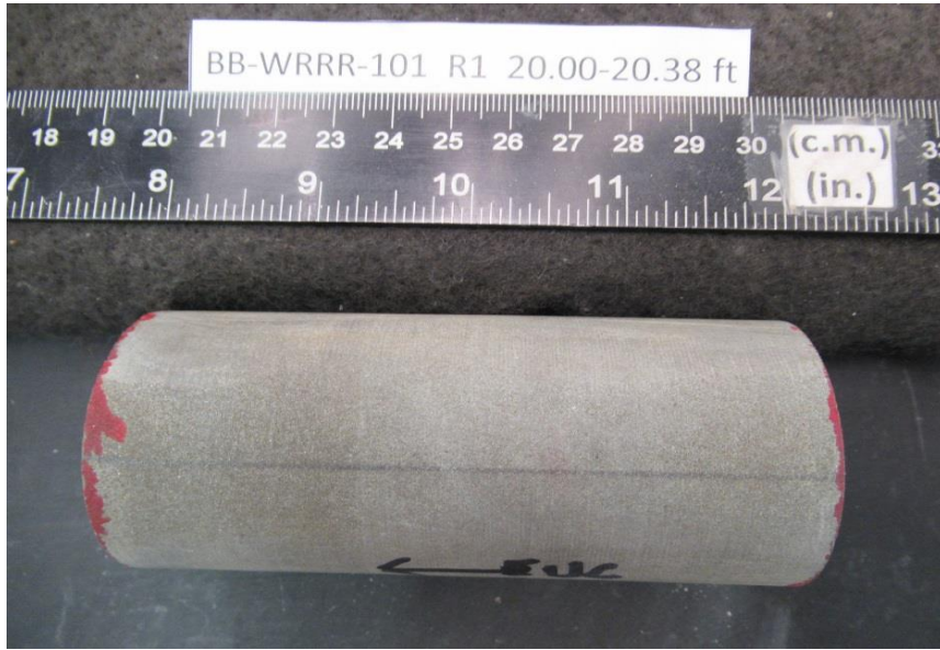
After cutting and grinding
