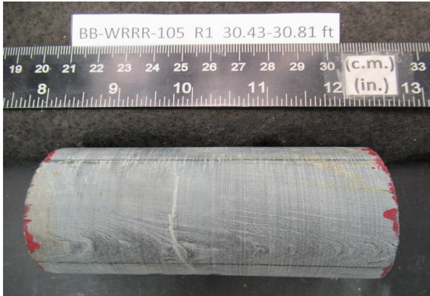
After cutting and grinding
