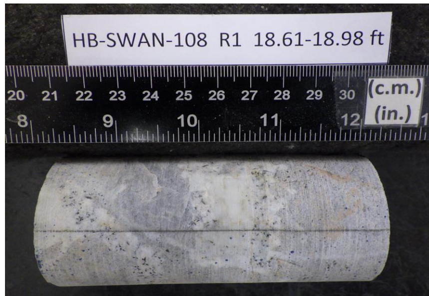
After cutting and grinding
