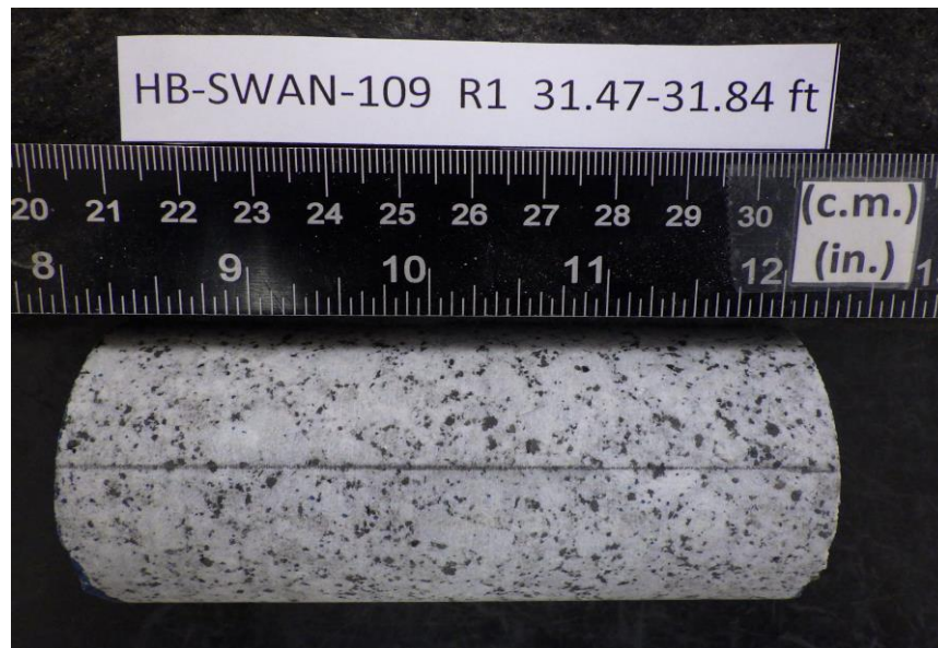
After cutting and grinding
