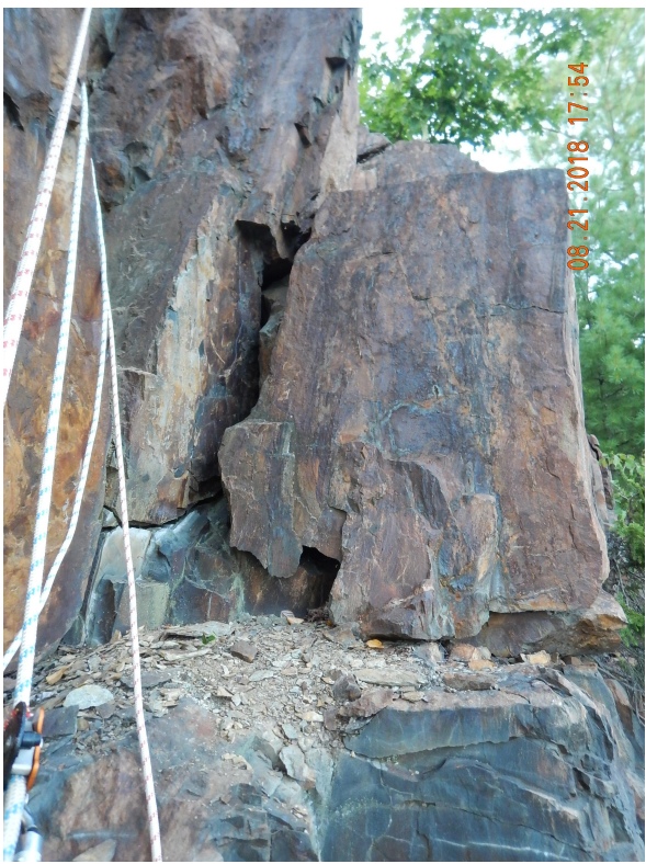
PHOTO 2 (RIGHT): SIDE VIEW LOOKING NORTH WITH OPEN BACK AND BASAL JOINTS VISIBLE.
