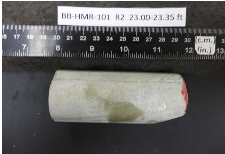
After cutting and grinding
