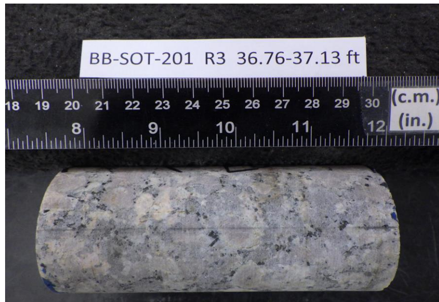
After cutting and grinding
