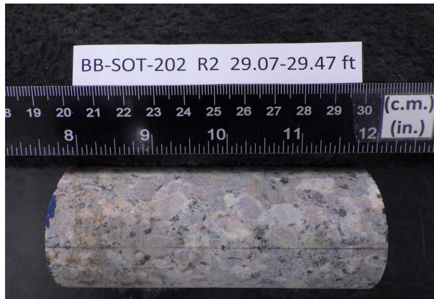
After cutting and grinding
