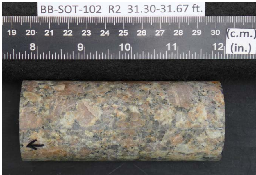
After cutting and grinding
