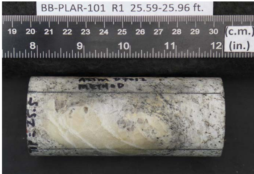
After cutting and grinding
