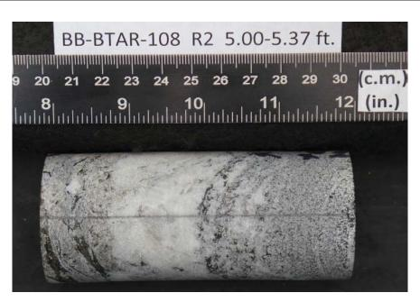
After cutting and grinding
