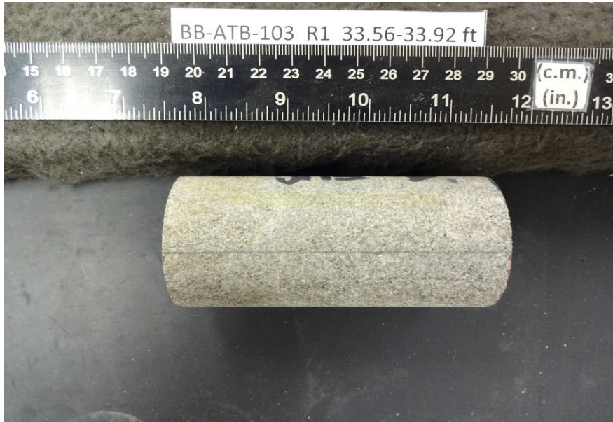
After cutting and grinding
