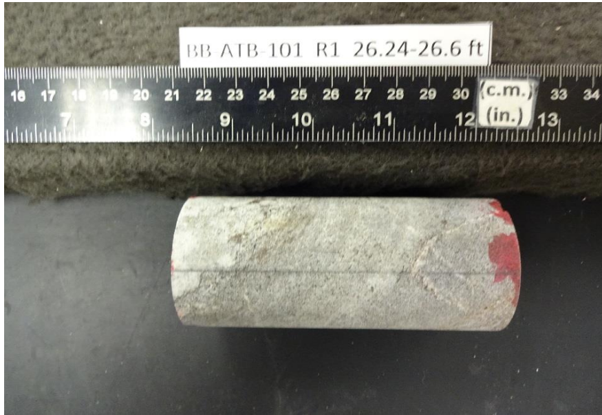
After cutting and grinding
