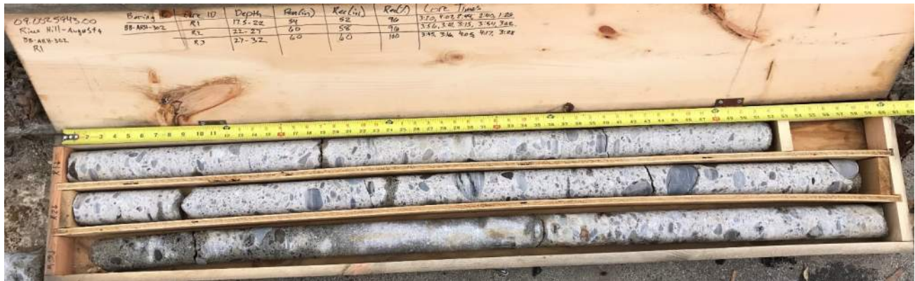
Cored Concrete, North Abutment (BB-ARH-302)
