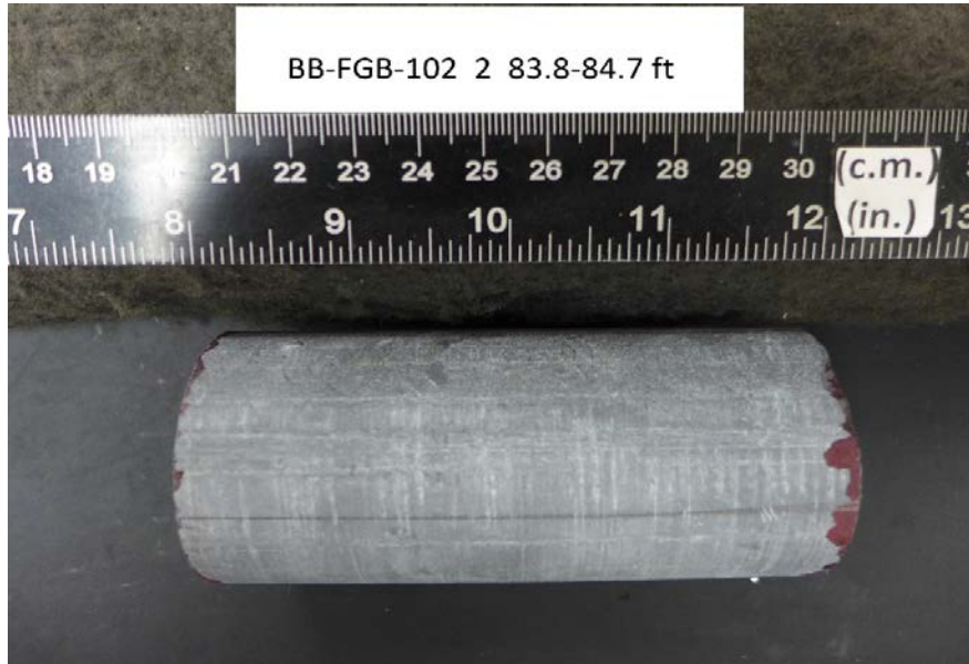
After cutting and grinding
