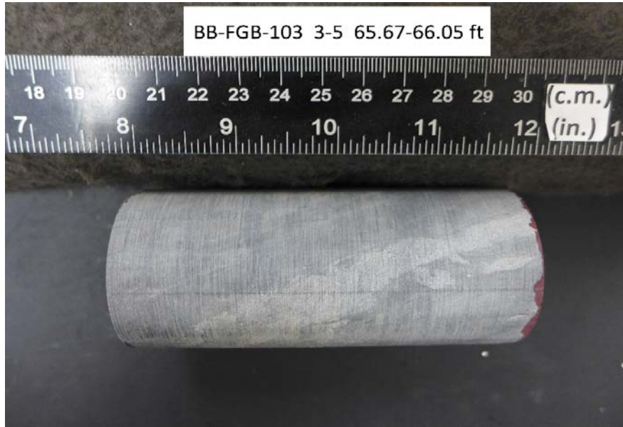
After cutting and grinding
