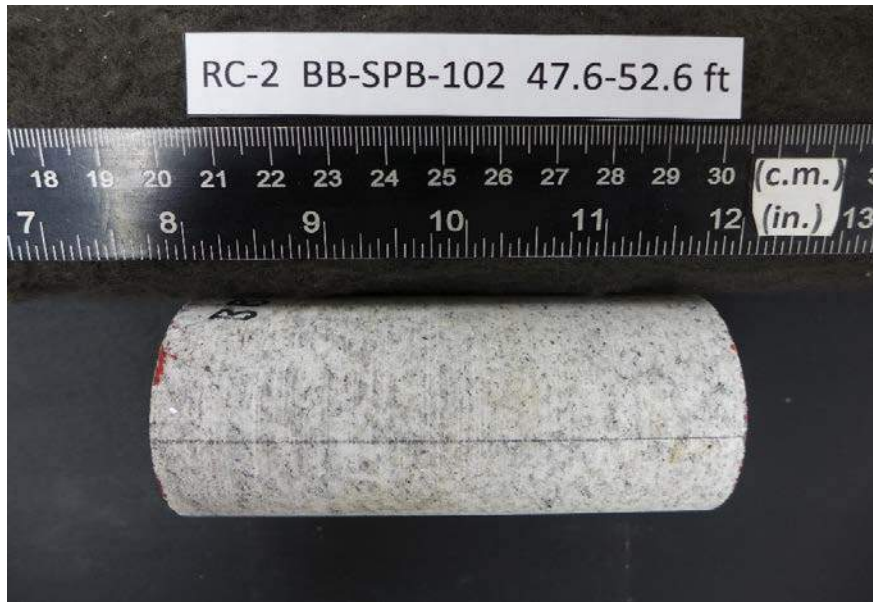
After cutting and grinding
