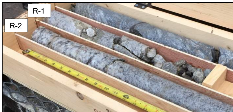
Photo 3: Boring BB-SPB-102: Rock Core Samples R-1 (Row 2), R-2 (Row 3). Note: Row 1 contains a rock core from a separate project.
