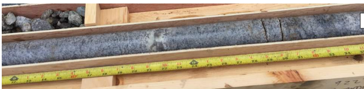
Photo 4: Boring BB-SPB-102: Rock Core Samples R-2 (middle).
