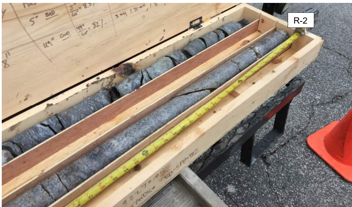
Photo 5: Boring BB-SPB-102: Rock Core Samples R-2 (End).
