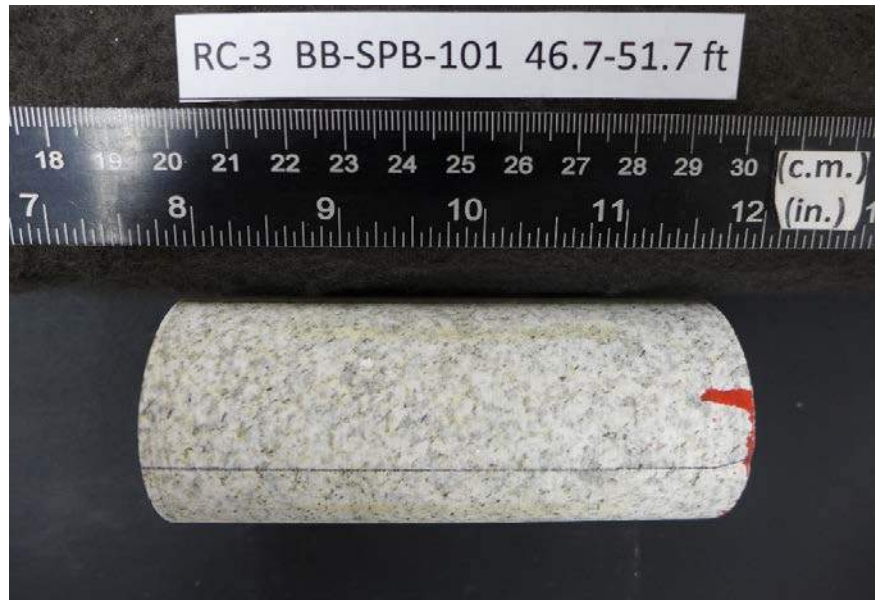
After cutting and grinding
