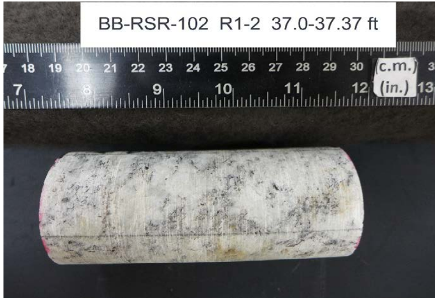
After cutting and grinding
