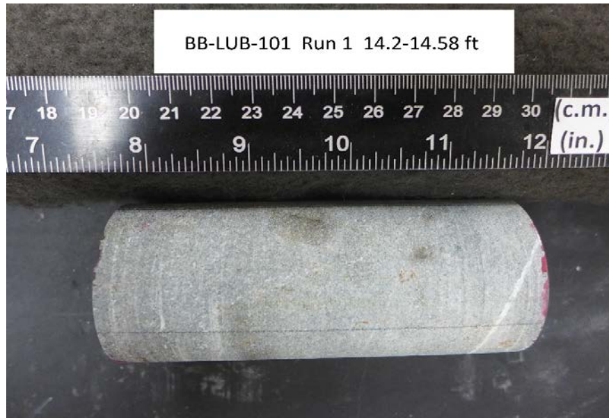
After cutting and grinding
