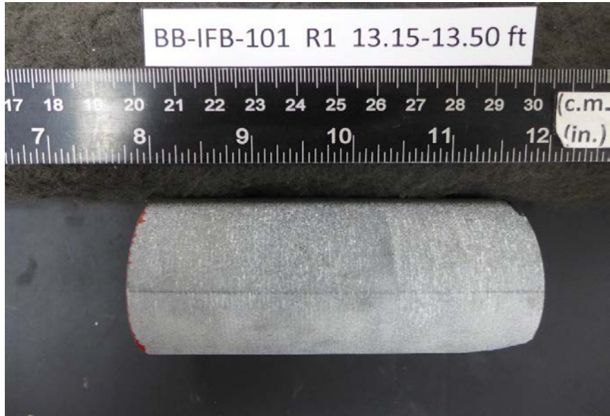
After cutting and grinding
