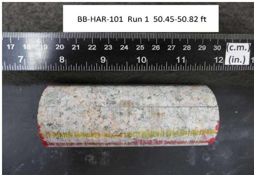
After cutting and grinding
