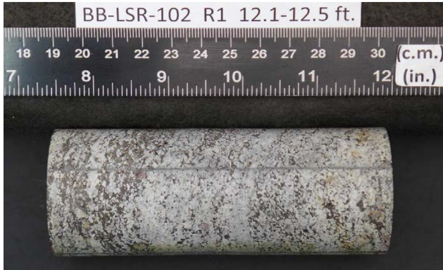
After cutting and grinding
