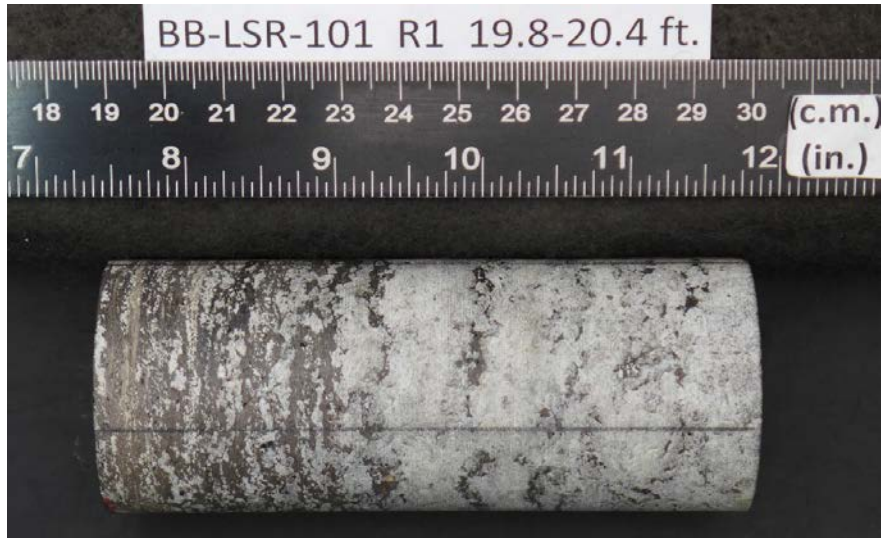
After cutting and grinding
