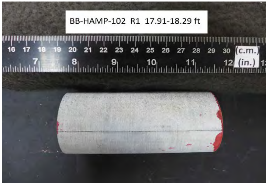
After cutting and grinding
