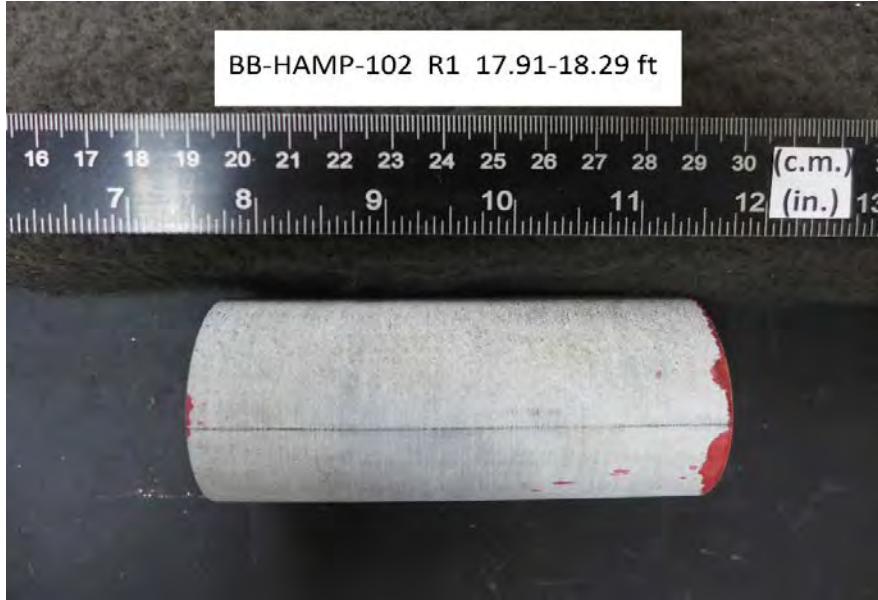
After cutting and grinding
