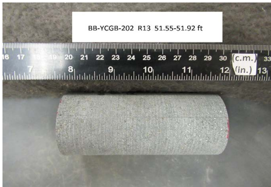
After cutting and grinding
