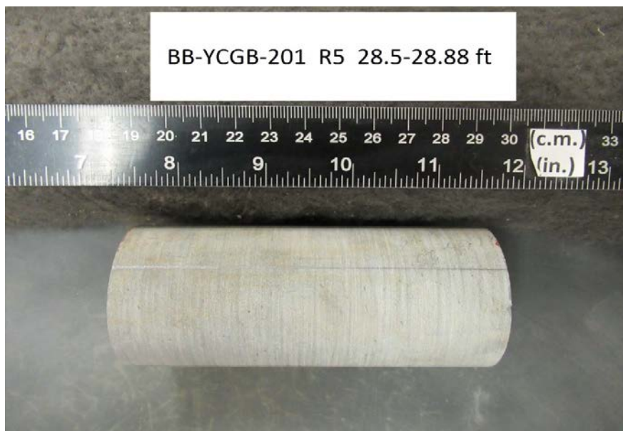
After cutting and grinding
