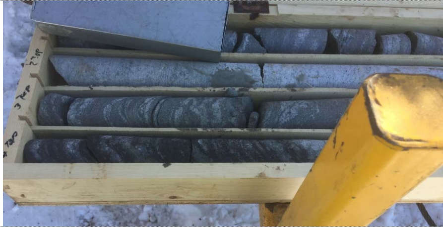
Photo 1: Boring BB-TNR-105 Rock Core Samples R-1 (Row 3) and R-2 (Row 4); top sections of each sample.
