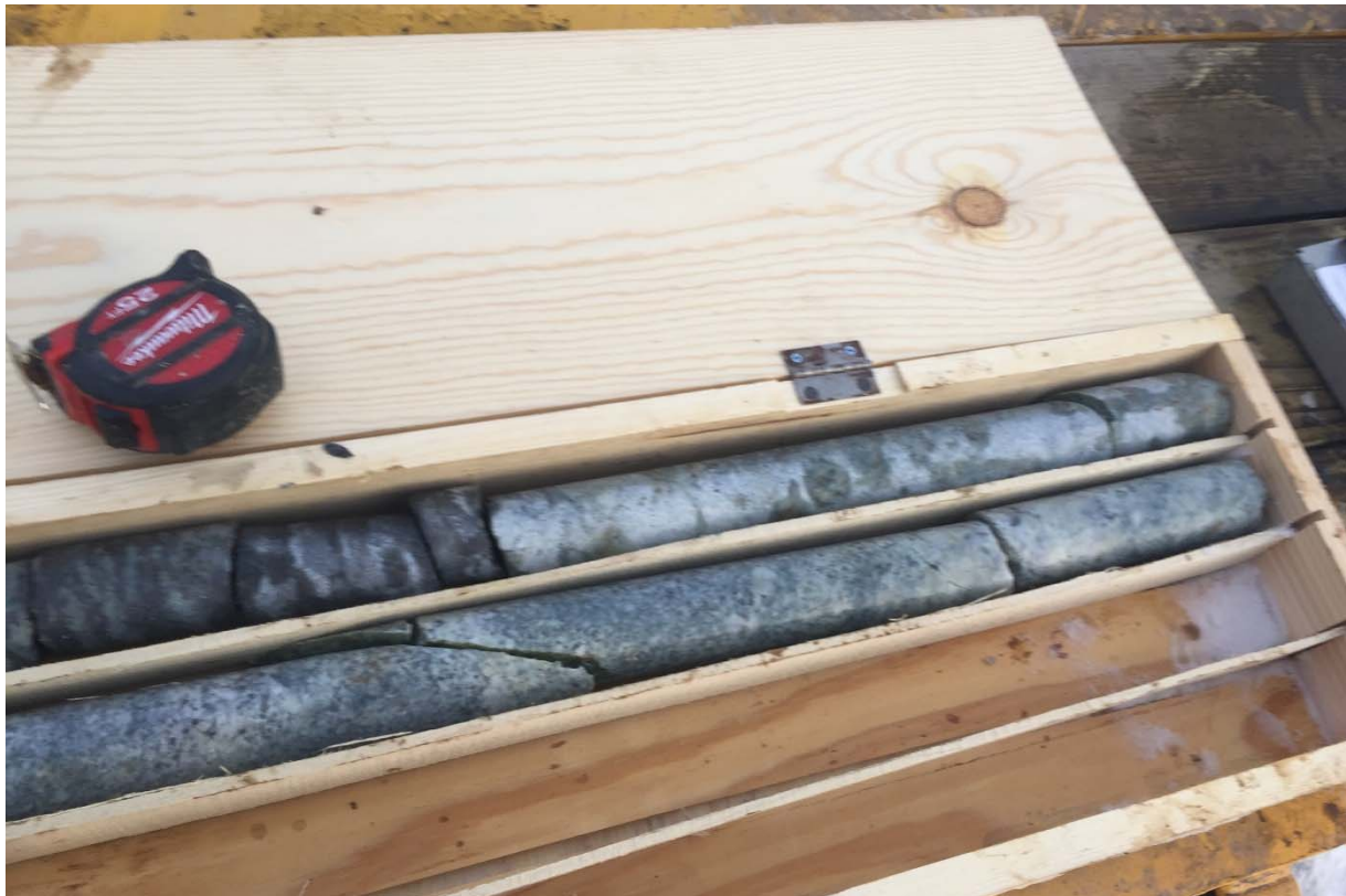
Photo 3: Boring BB-TNR-103 Rock Core Samples R-1 (Row 1) and R-2 (Row 2); bottom sections of each sample.
