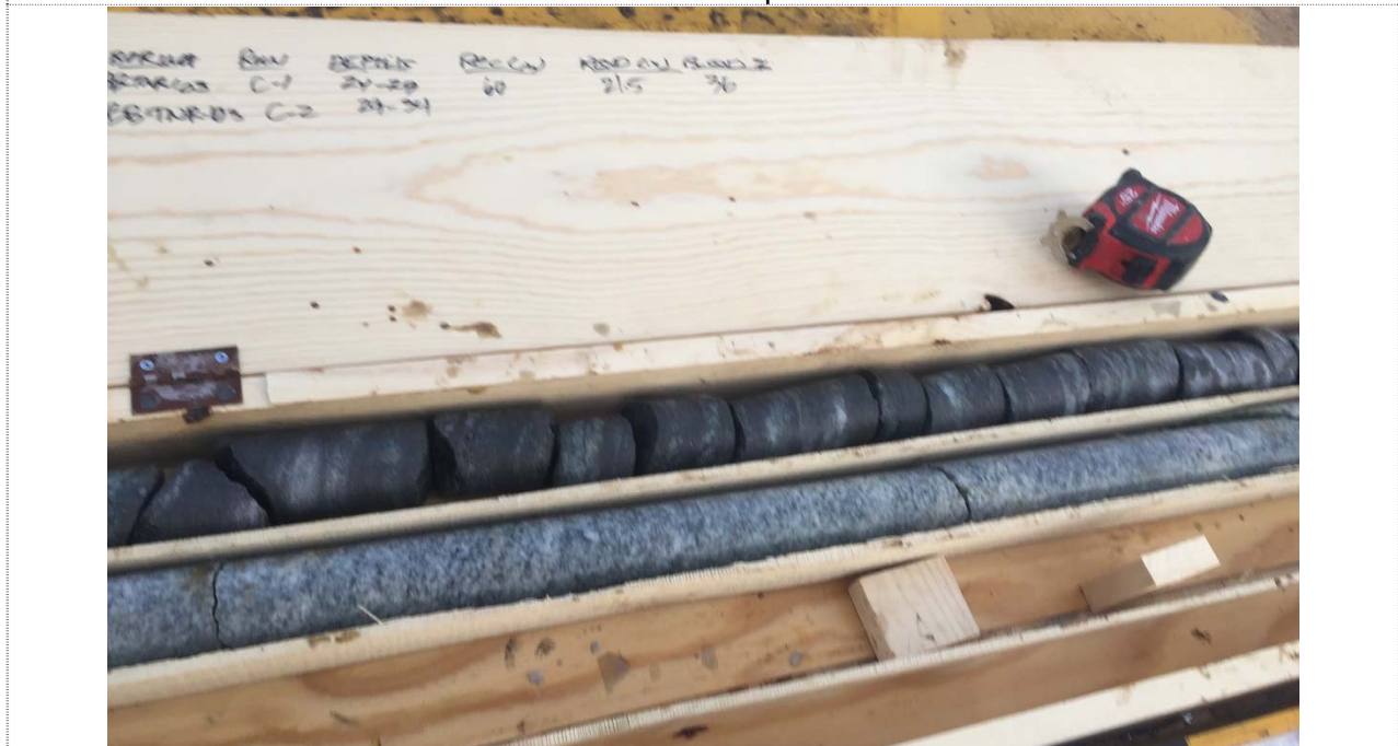
Photo 2: Boring BB-TNR-103 Rock Core Samples R-1 (Row 1) and R-2 (Row 2); mid sections of each sample.
