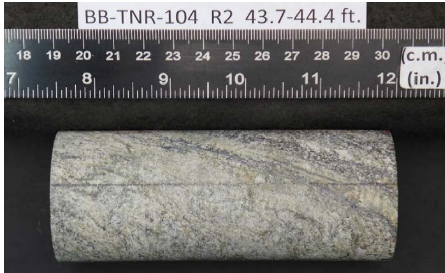
After cutting and grinding
