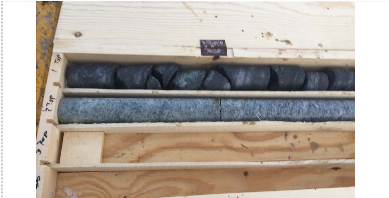
Photo 1: Boring BB-TNR-103 Rock Core Samples R-1 (Row 1) and R-2 (Row 2); top sections of each sample.
