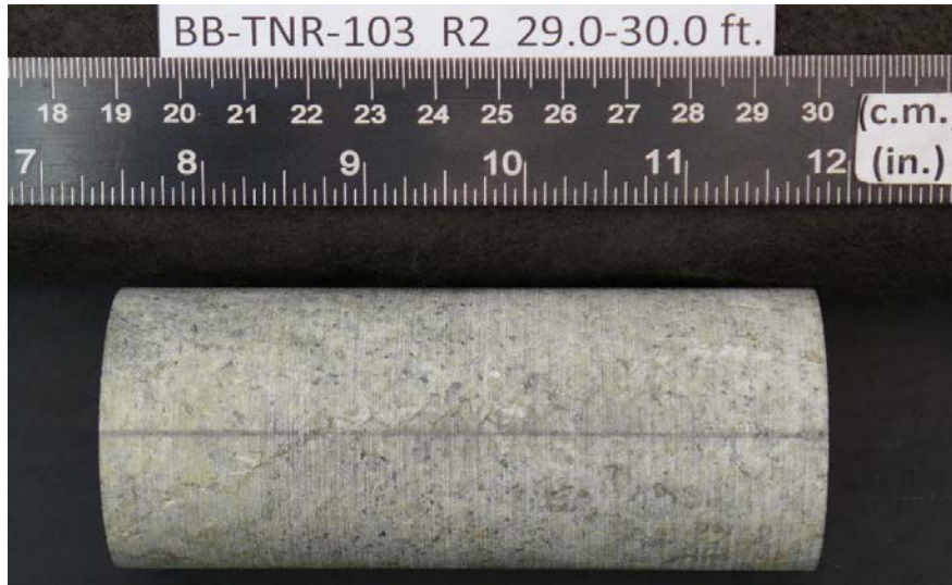
After cutting and grinding
