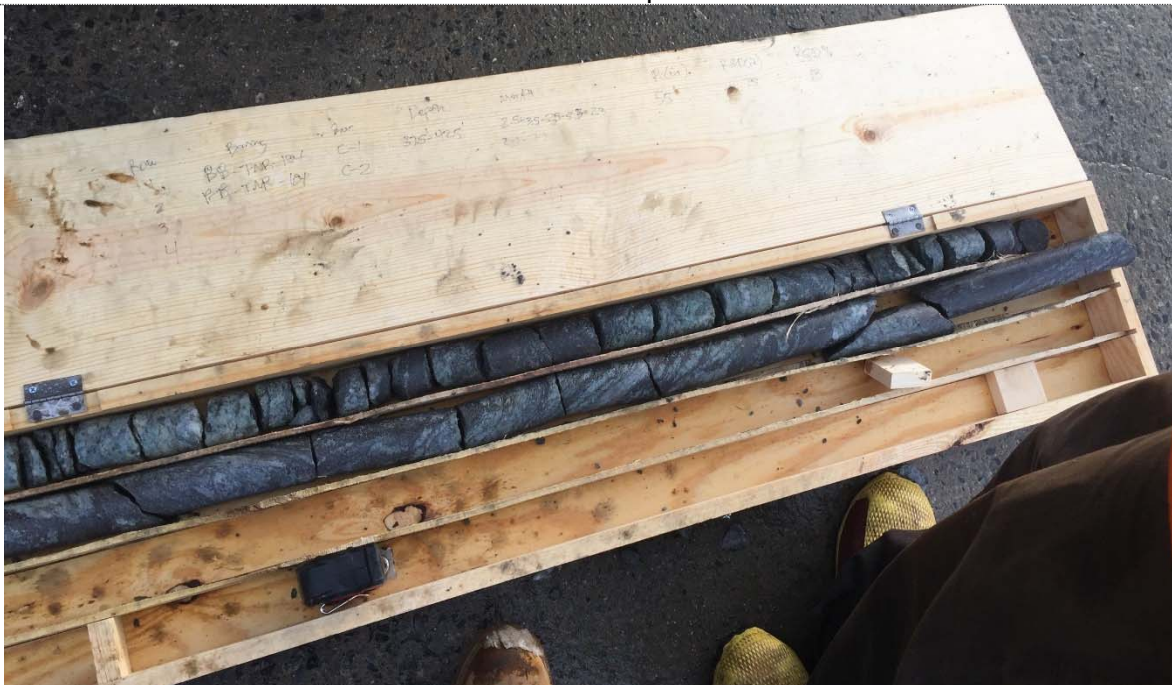
Photo 2: Boring BB-TNR-104 Rock Core Samples R-1 (Row 1) and R-2 (Row 2); mid to bottom sections of each sample.
