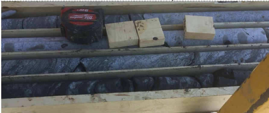
Photo 3: Boring BB-TNR-105 Rock Core Samples R-1 (Row 3) and R-2 (Row 4); mid to bottom sections of each sample.
