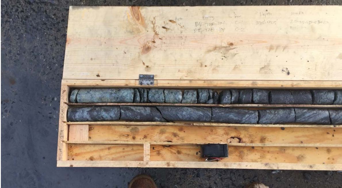
Photo 1: Boring BB-TNR-104 Rock Core Samples R-1 (Row 1) and R-2 (Row 2); top sections of each sample.
