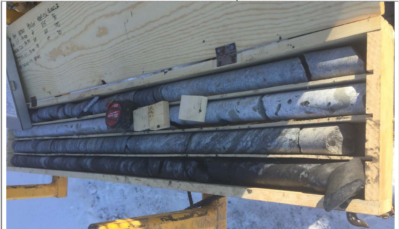
Photo 5: Boring BB-TNR-105 Rock Core Samples R-1 (Row 3) and R-2 (Row 4); entire sections of each sample.
