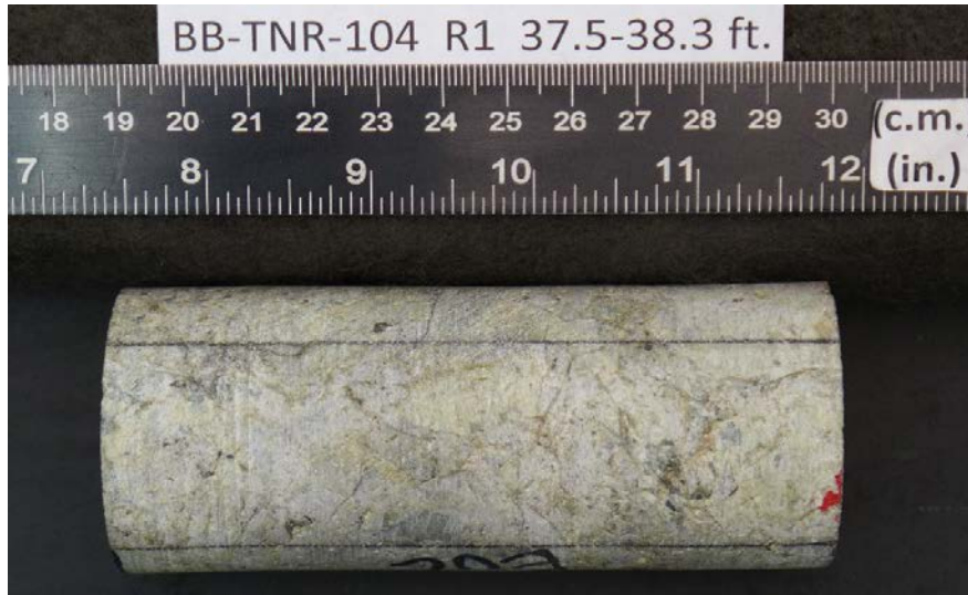
After cutting and grinding
