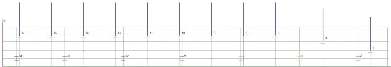
FB-MultiPier model of abutment and piles corresponding with record plan piles (below)
