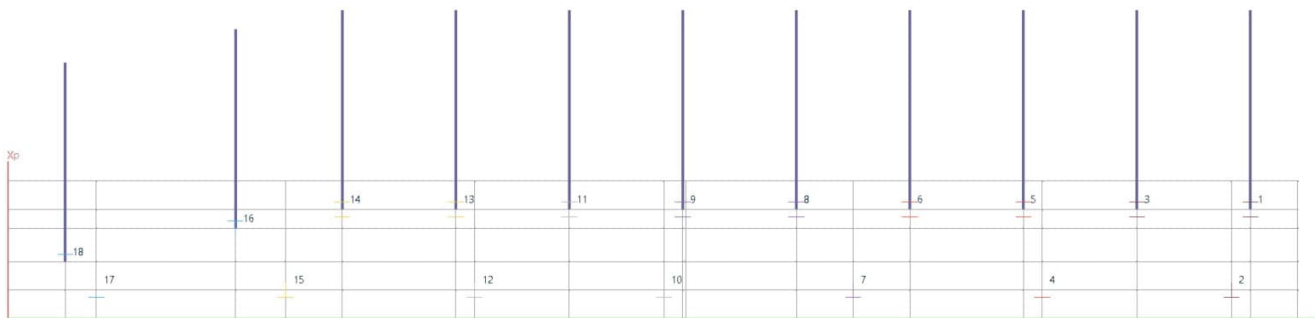
FB-MultiPier model of abutment and piles corresponding with record plan piles (below)
