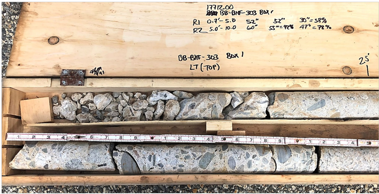
Core box containing dried core (H size) from test boring BB-BHF-303 (Box 1 of 3); left side of core box (top portion of cores). Slots from top to bottom: 1) R1; 2) R2.
