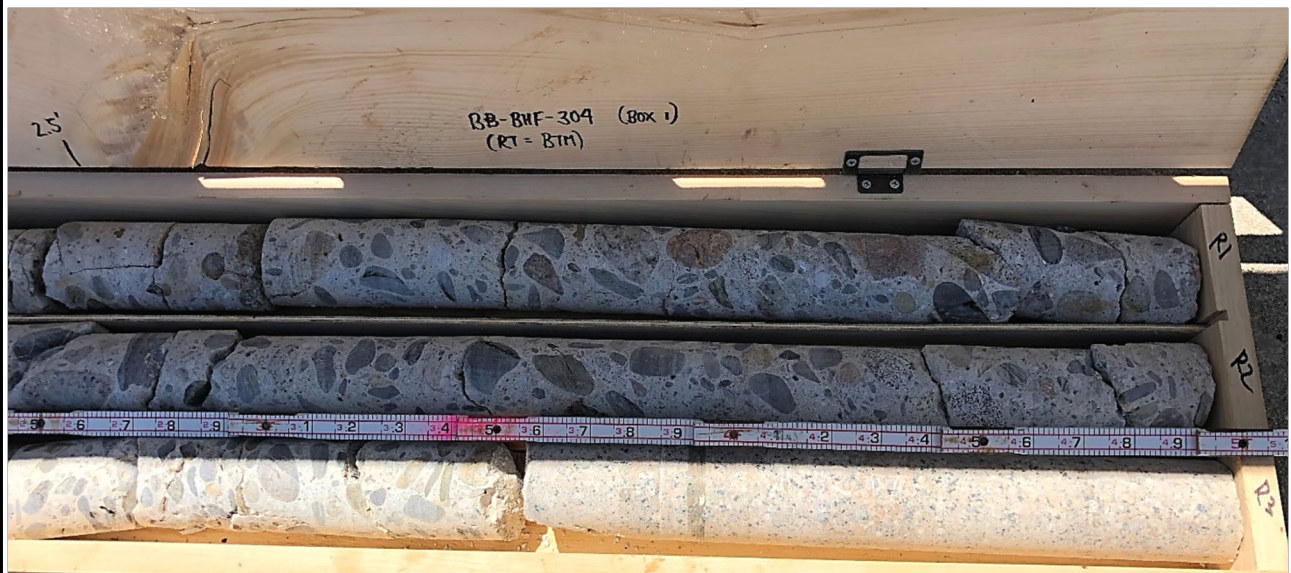
Core box containing dried core (H size) from test boring BB-BHF-304 (Box 1 of 3); right side of core box (bottom portion of cores). Slots from top to bottom:
