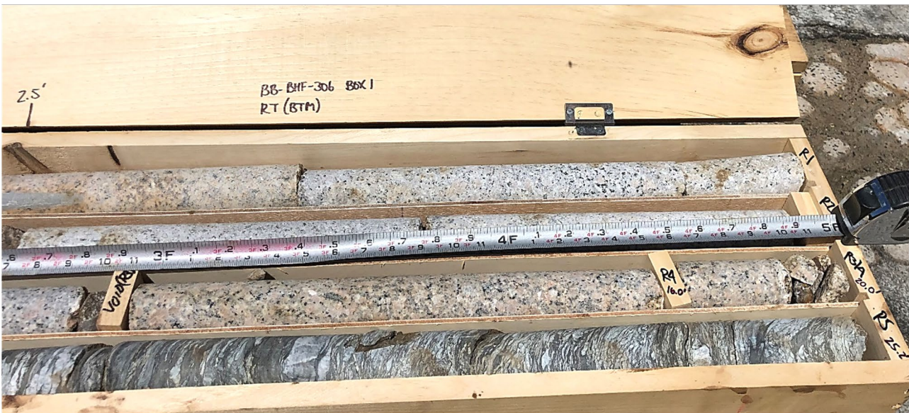
Core box containing dried core from test boring BB-BHF-306 (Box 1 of 2); right side of core box (bottom portion of cores). Slots from top to bottom:
