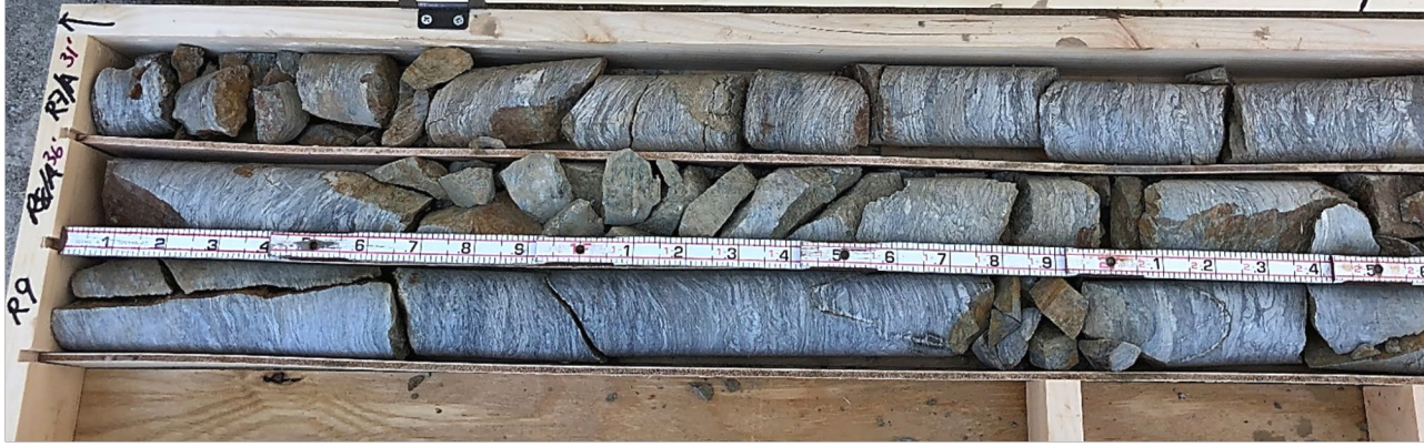
Core box containing dried core from test boring BB-BHF-304 (Box 3 of 3); left side of core box (top portion of cores). Slots from top to bottom:
