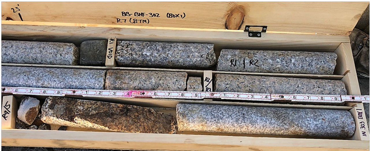
Core box containing dried core (H size) from test boring BB-BHF-302 (Box 1 of 3); right side of core box (bottom portion of cores). Slots from top to bottom:
