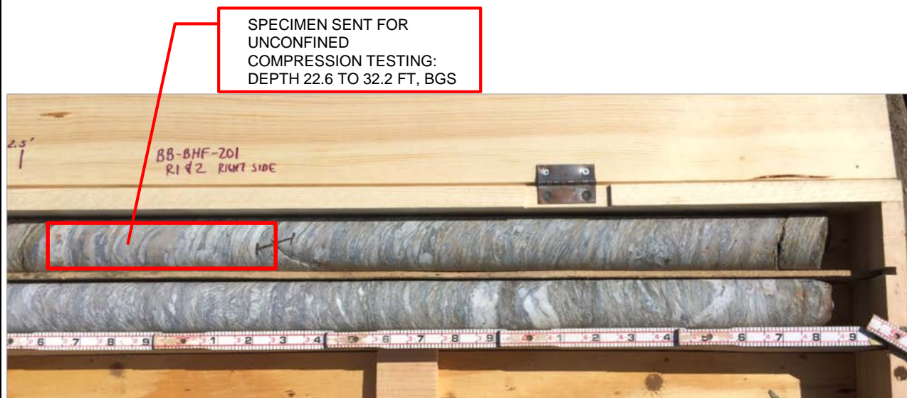
Photo 2: Core box containing dried core from test boring BB-BHF-201: Right side of core box (bottom 2.5-foot portion of cores).
