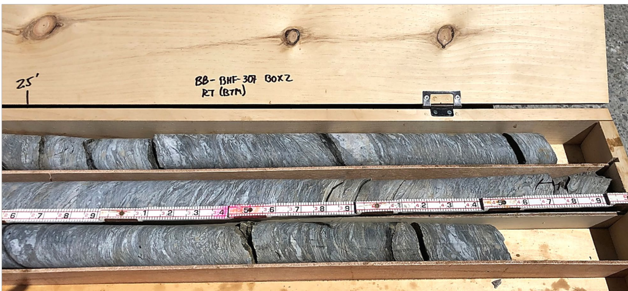
Core box containing dried core from test boring BB-BHF-307 (Box 2 of 2); right side of core box (bottom portion of cores). Slots from top to bottom:
