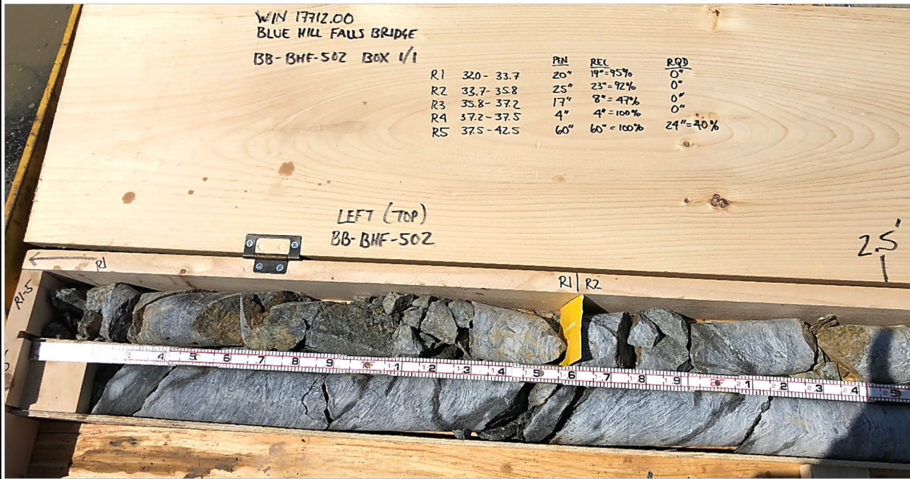
Core box containing dried core from test boring BB-BHF-502 (Box 1 of 1); left side of core box (top portion of cores). Slots from top to bottom:
