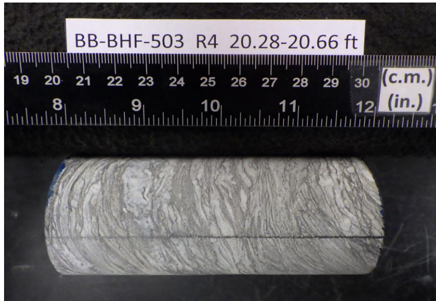
After cutting and grinding
