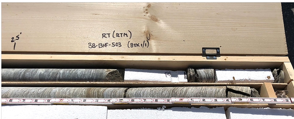
Core box containing dried core from test boring BB-BHF-503 (Box 1 of 1); right side of core box (bottom portion of cores). Slots from top to bottom:
