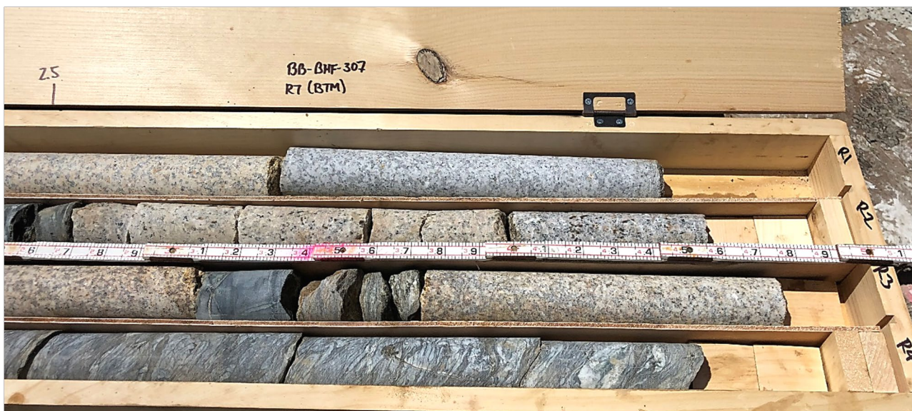
Core box containing dried core from test boring BB-BHF-307 (Box 1 of 2); right side of core box (bottom portion of cores). Slots from top to bottom:
