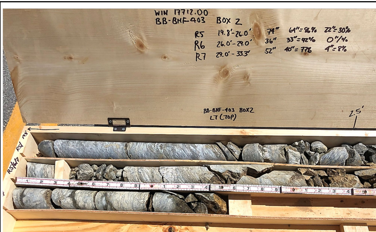
Core box containing dried core from test boring BB-BHF-403 (Box 2 of 2); left side of core box (top portion of cores). Slots from top to bottom:
