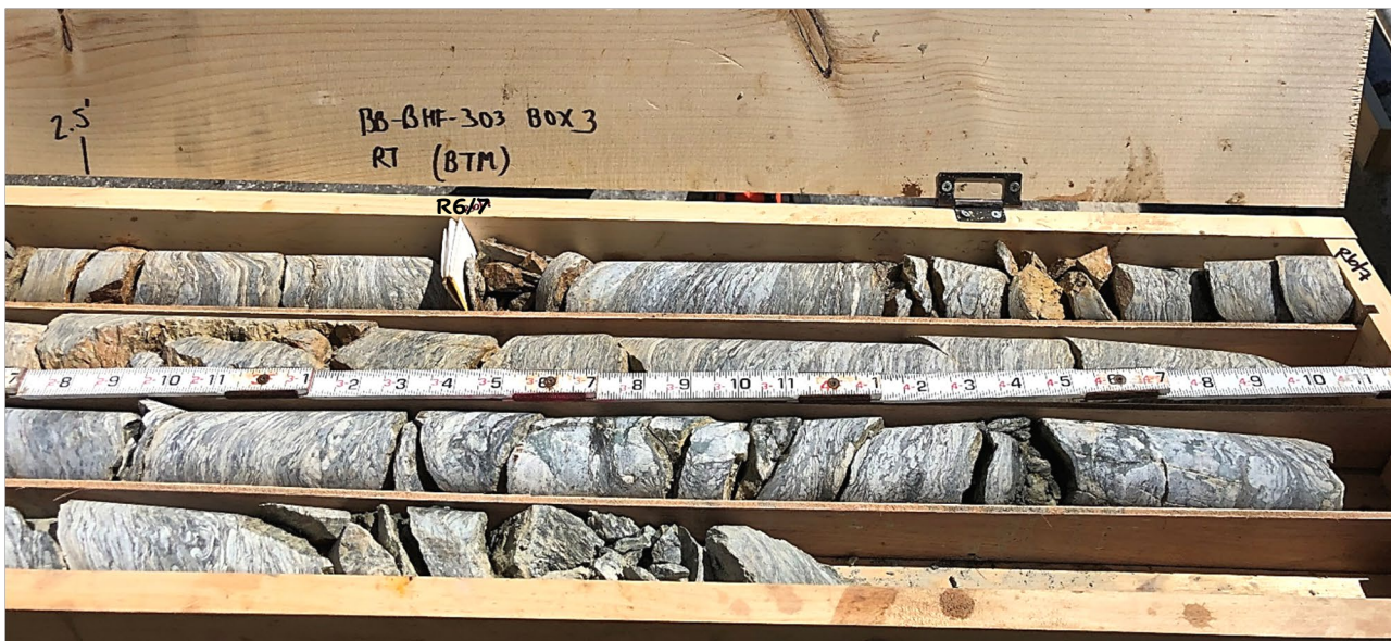
Core box containing dried core from test boring BB-BHF-303 (Box 3 of 3); right side of core box (bottom portion of cores). Slots from top to bottom:
