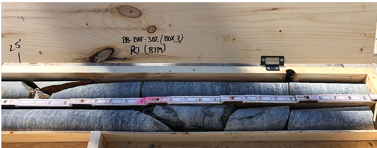
Core box containing dried core from test boring BB-BHF-302 (Box 3 of 3); right side of core box (bottom portion of cores). Slots from top to bottom:
