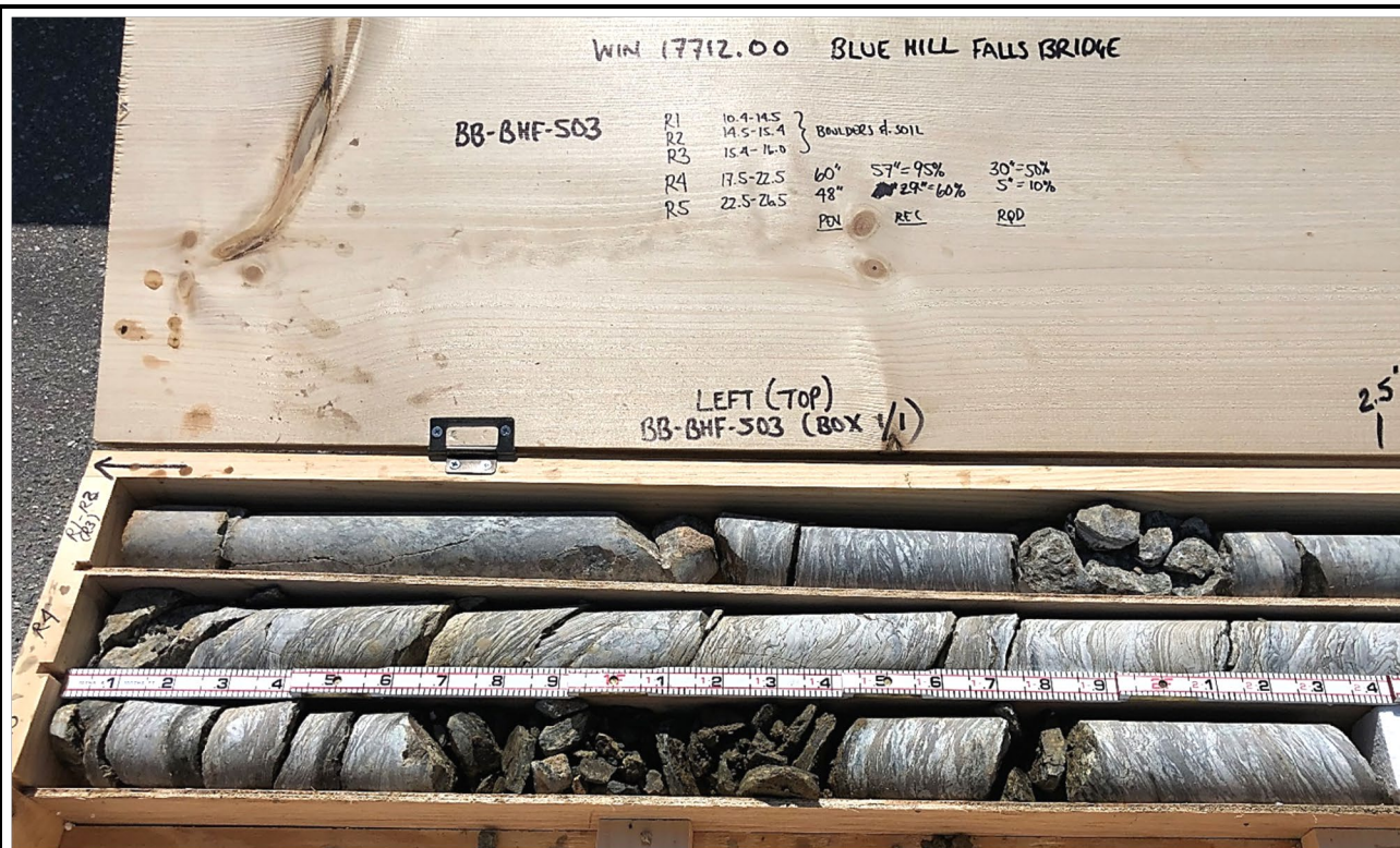
Core box containing dried core from test boring BB-BHF-503 (Box 1 of 1); left side of core box (top portion of cores). Slots from top to bottom:
