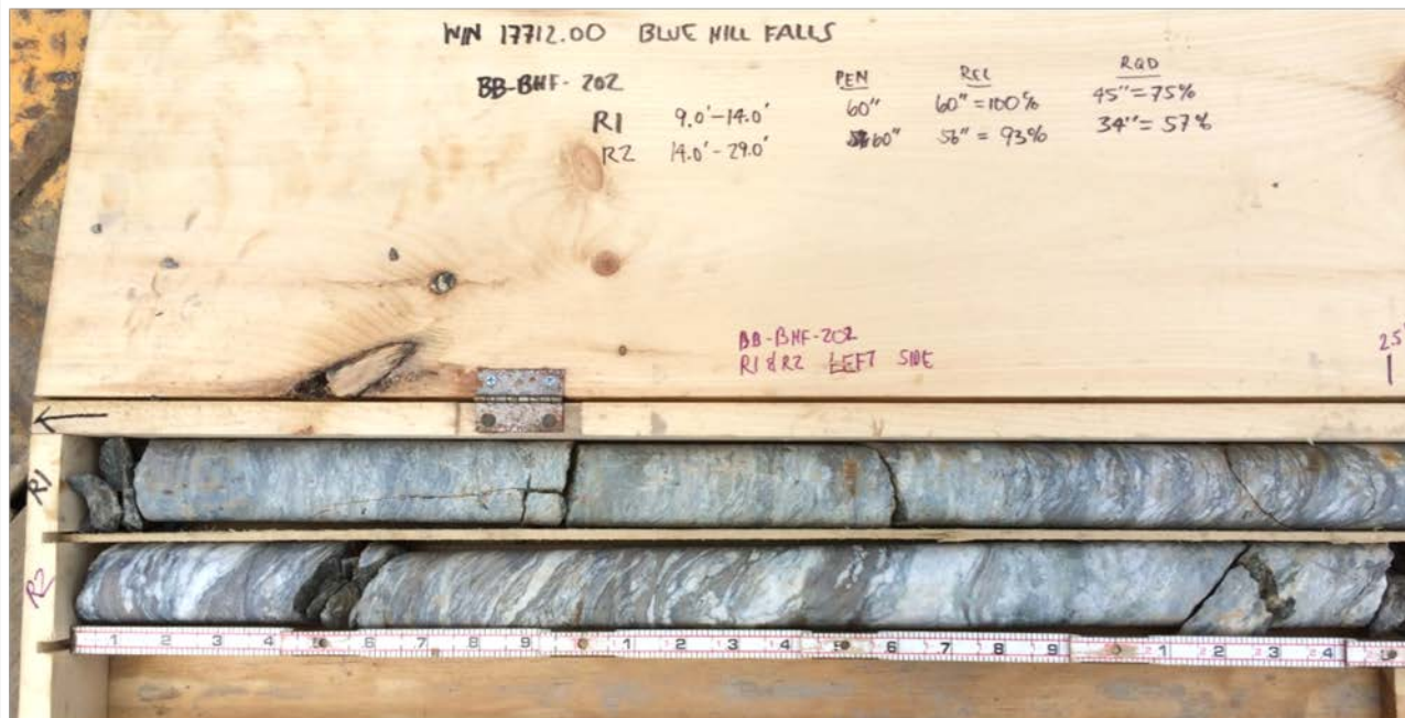
Photo 5: Core box containing dried core from test boring BB-BHF-202:
