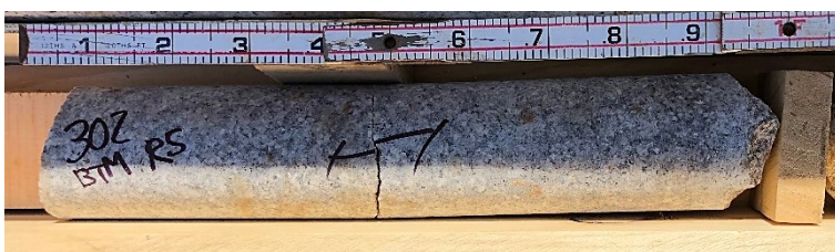
Core (H-size) from test boring BB-BHF-302 – bottom piece of R5.
