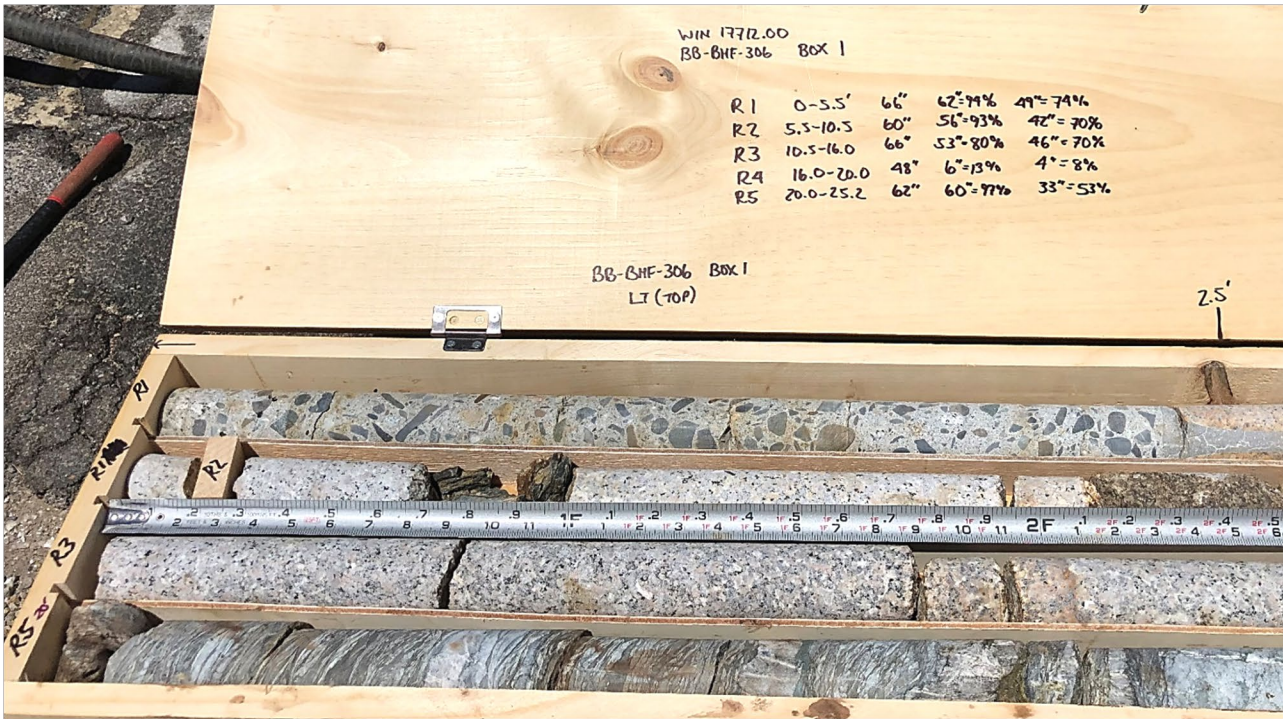
Core box containing dried core from test boring BB-BHF-306 (Box 1 of 2); left side of core box (top portion of cores). Slots from top to bottom:
