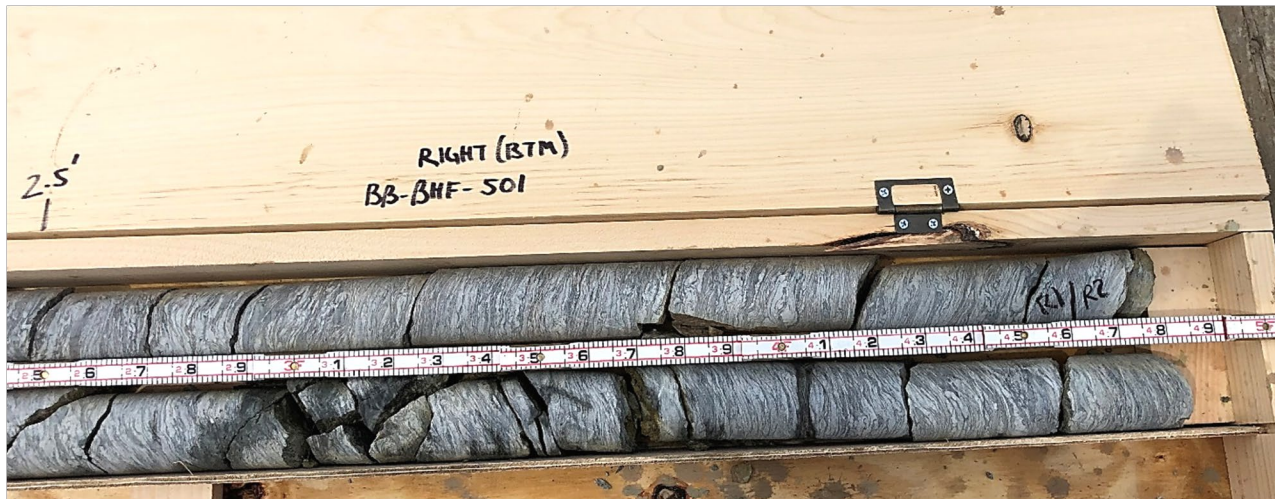
Core box containing dried core from test boring BB-BHF-501 (Box 1 of 1); right side of core box (bottom portion of cores). Slots from top to bottom:
