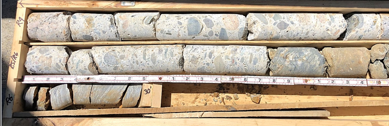
Core box containing dried core from test boring BB-BHF-304 (Box 2 of 3); left side of core box (top portion of cores). Slots from top to bottom:
