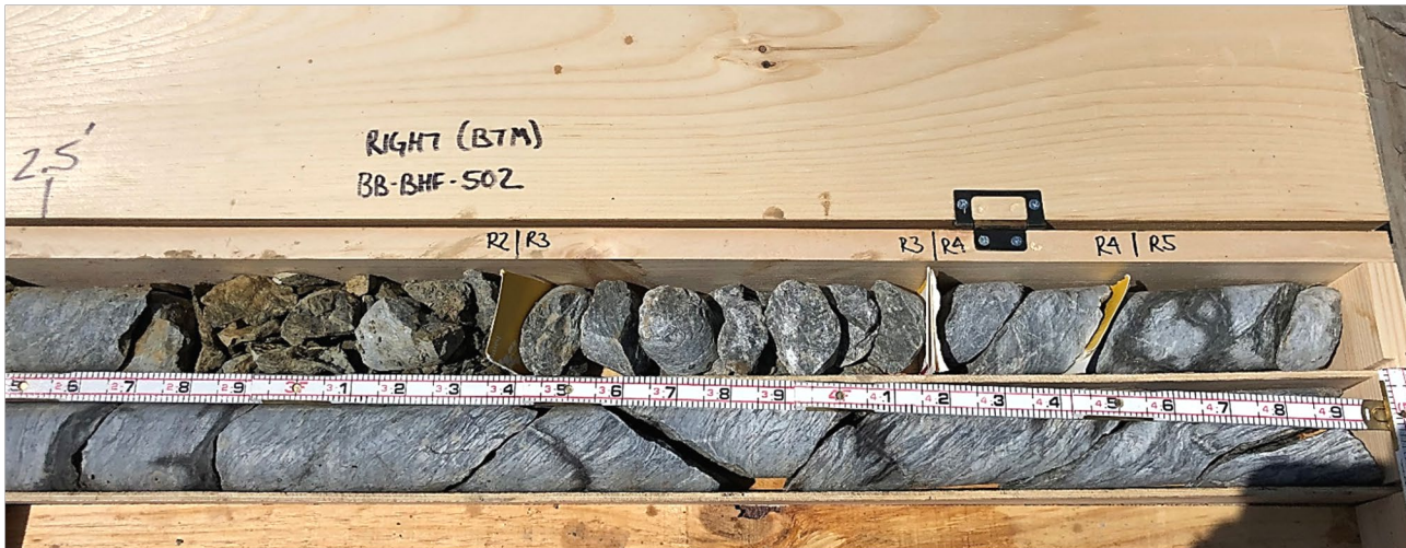
Core box containing dried core from test boring BB-BHF-502 (Box 1 of 1); right side of core box (bottom portion of cores). Slots from top to bottom:
