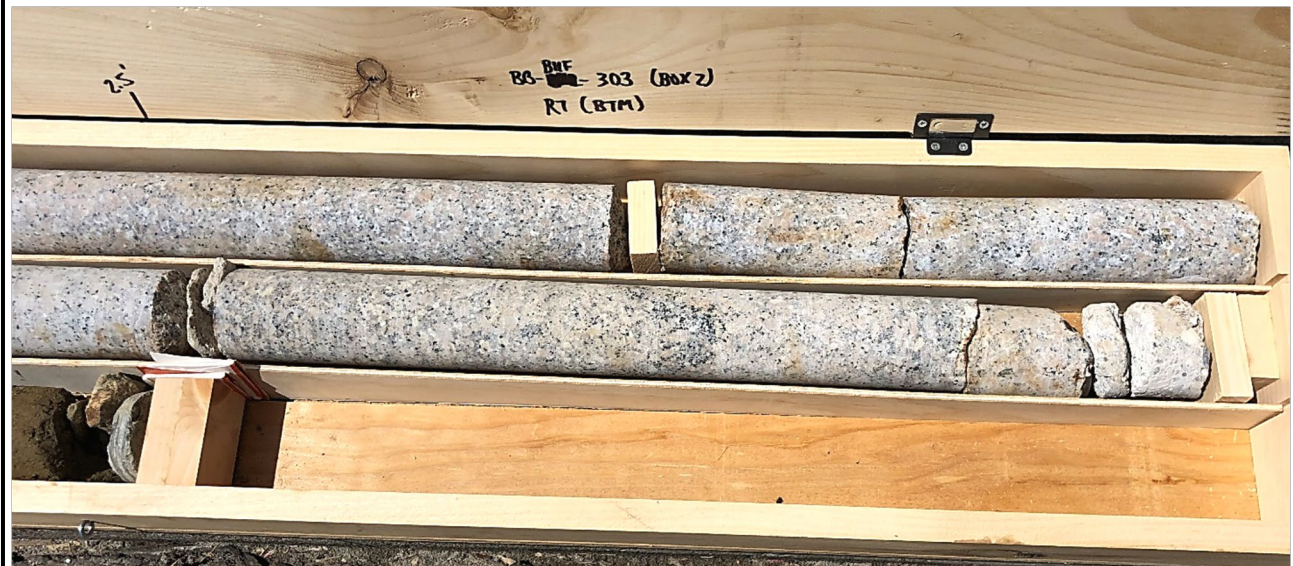
Core box containing dried core (H size) from test boring BB-BHF-303 (Box 2 of 3); right side of core box (bottom portion of cores). Slots from top to bottom:
