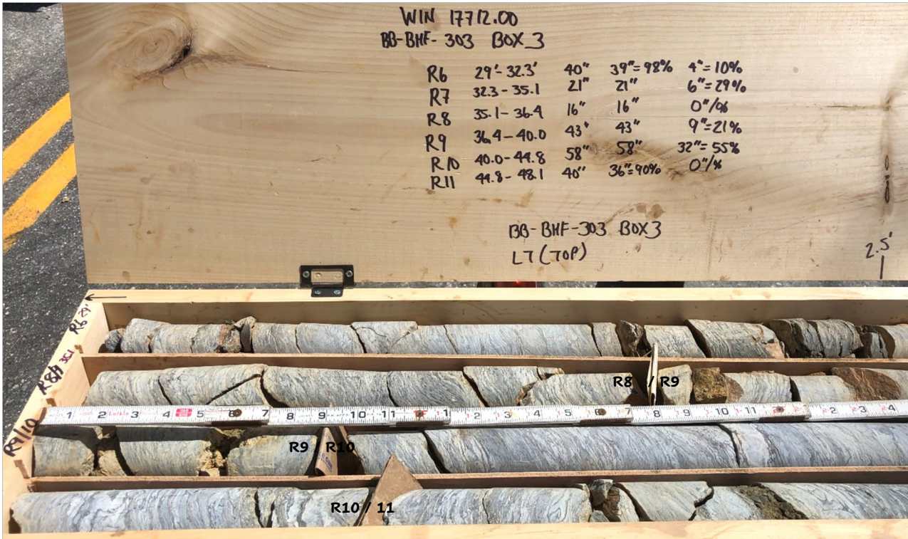
Core box containing dried core from test boring BB-BHF-303 (Box 3 of 3); left side of core box (top portion of cores). Slots from top to bottom:
