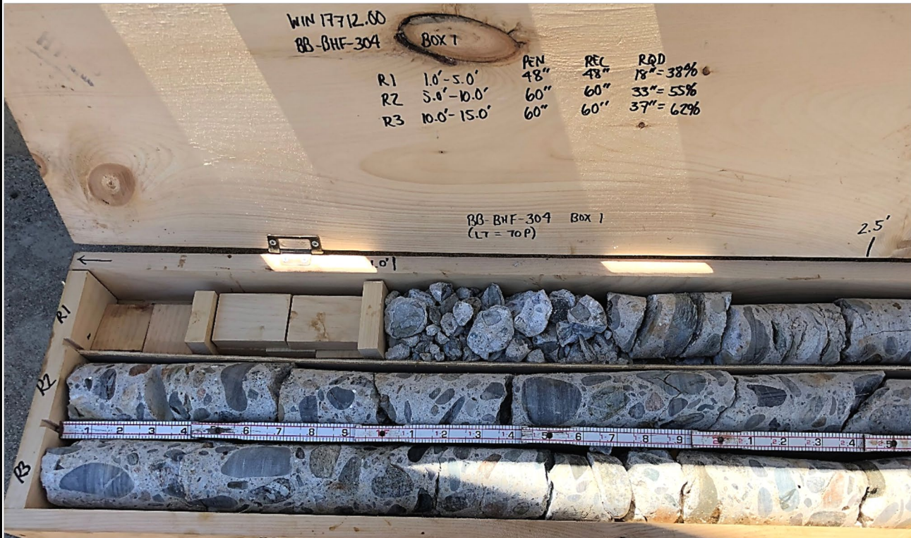
Core box containing dried core (H size) from test boring BB-BHF-304 (Box 1 of 3); left side of core box (top portion of cores). Slots from top to bottom:
