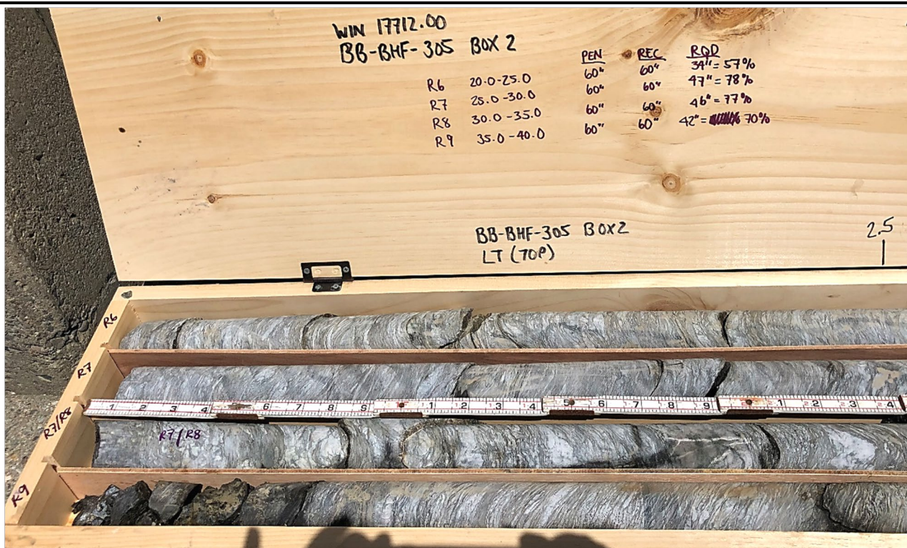
Core box containing dried core from test boring BB-BHF-305 (Box 2 of 2); left side of core box (top portion of cores).
