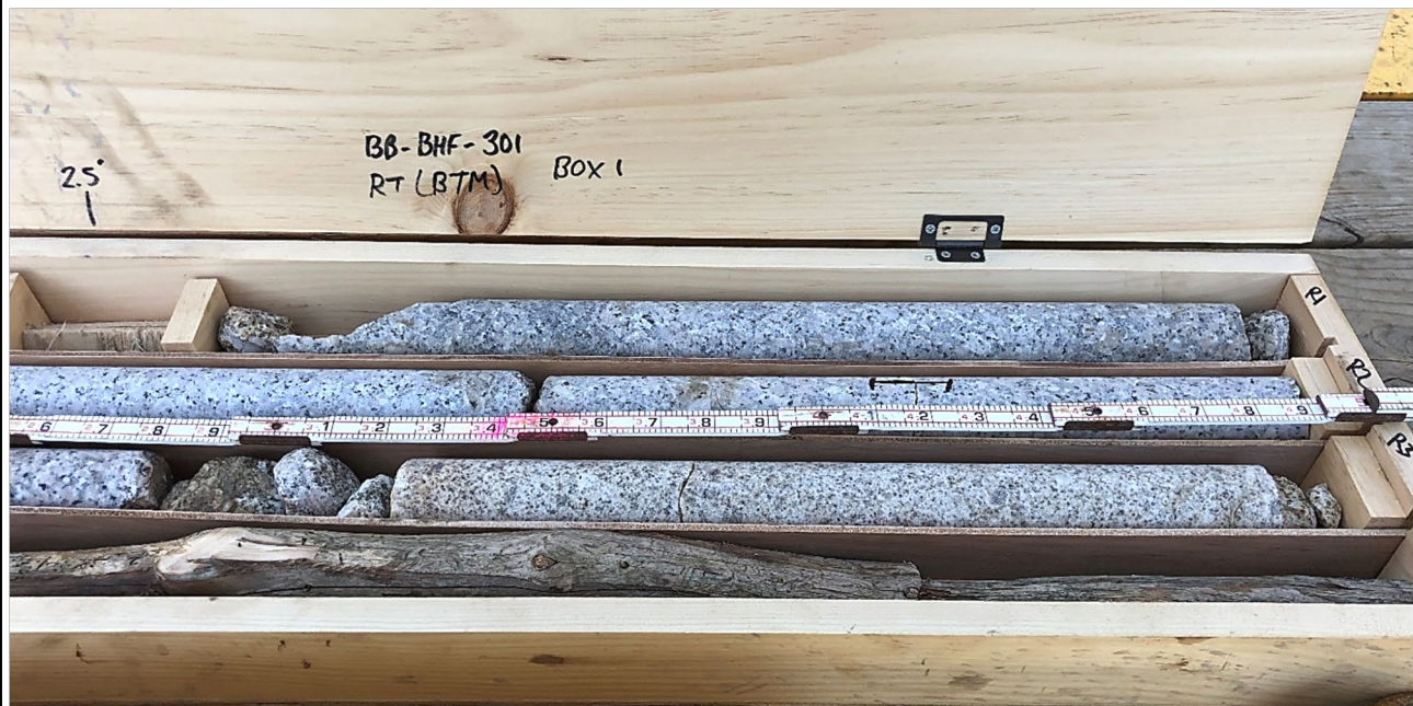
Core box containing dried core from test boring BB-BHF-301 (Box 1 of 1); right side of core box (bottom portion of cores). Slots from top to bottom:
