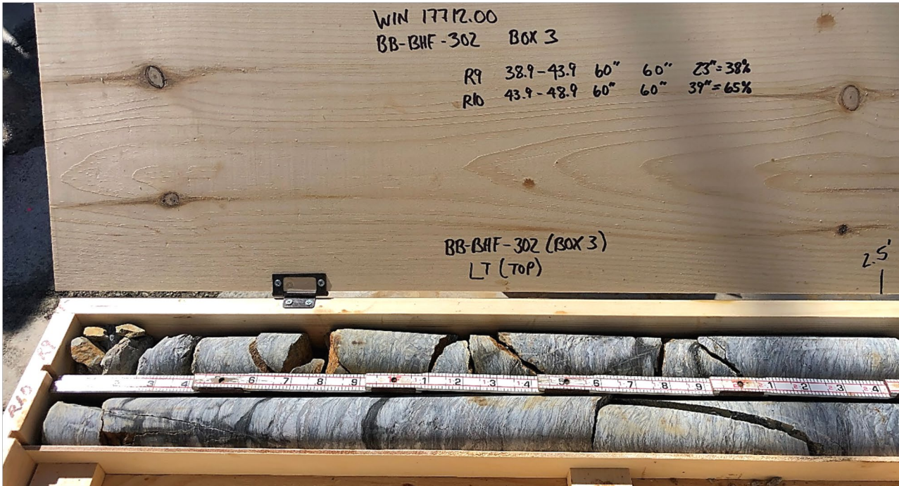
Core box containing dried core from test boring BB-BHF-302 (Box 3 of 3); left side of core box (top portion of cores). Slots from top to bottom:
