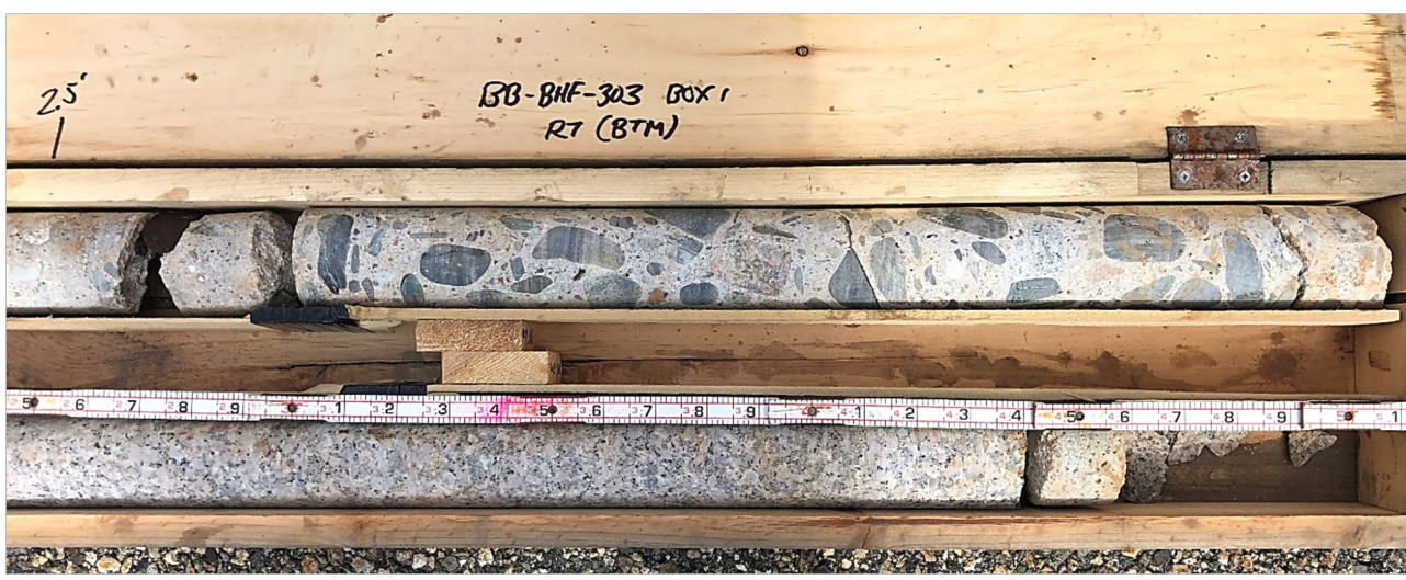
Core box containing dried core (H size) from test boring BB-BHF-303 (Box 1 of 3); right side of core box (bottom portion of cores). Slots from top to bottom: 1) R1; 2) R2.
