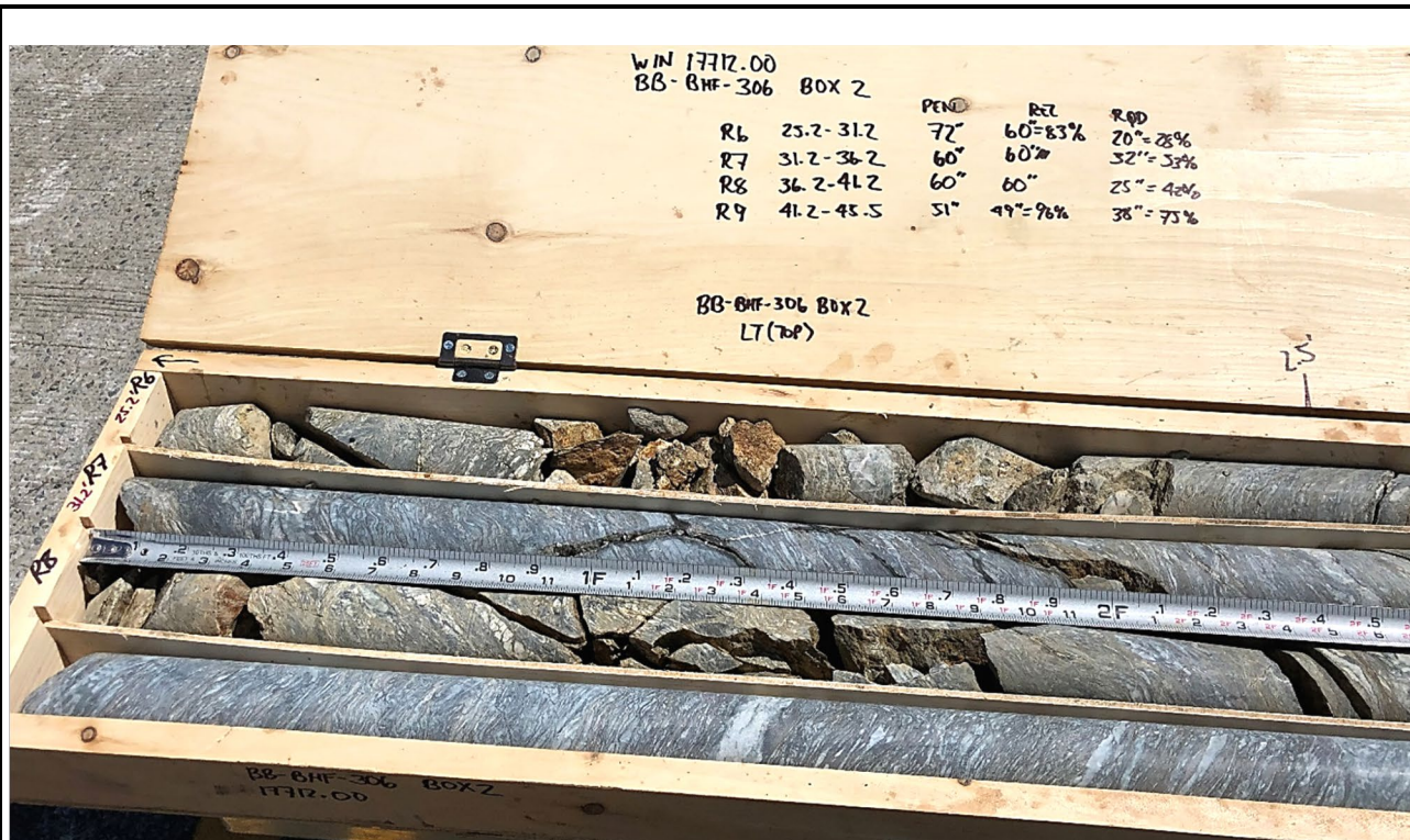
Core box containing dried core from test boring BB-BHF-306 (Box 2 of 2); left side of core box (top portion of cores). Slots from top to bottom:
