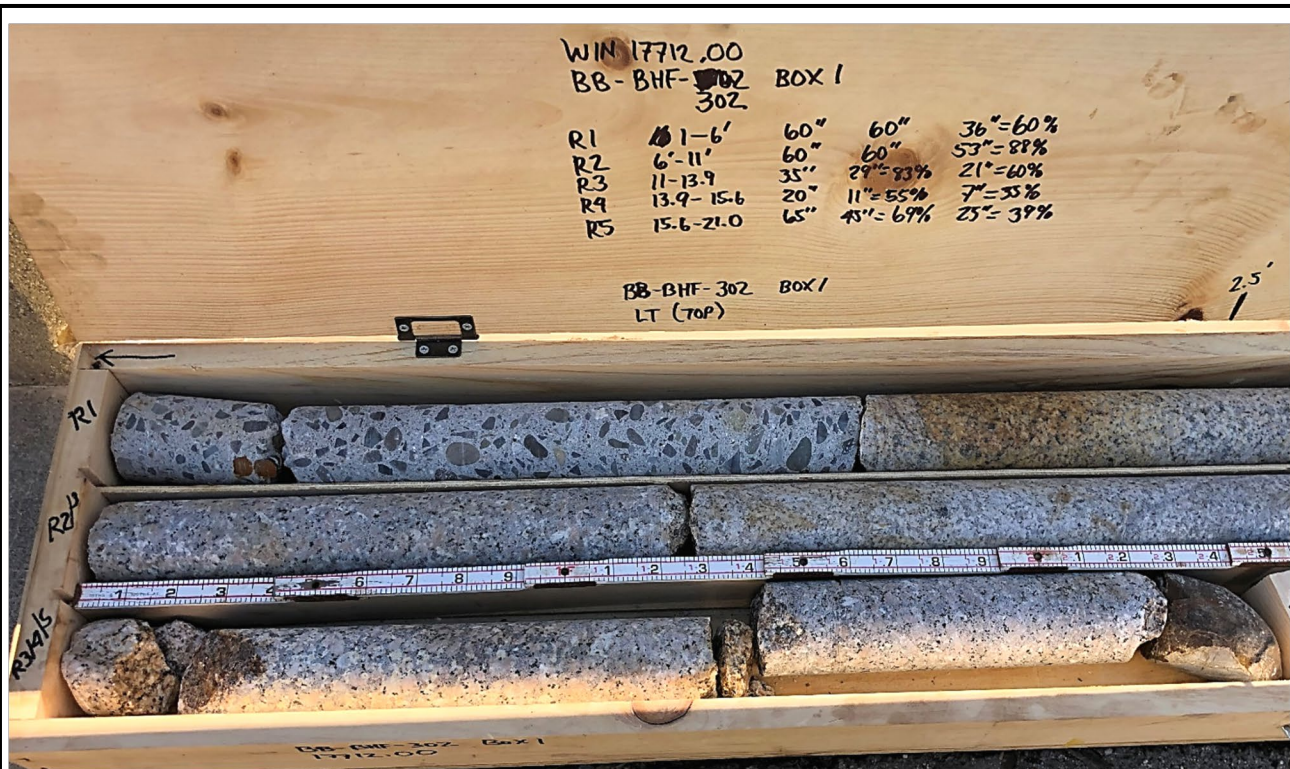
Core box containing dried core (H size) from test boring BB-BHF-302 (Box 1 of 3); left side of core box (top portion of cores). Slots from top to bottom:
