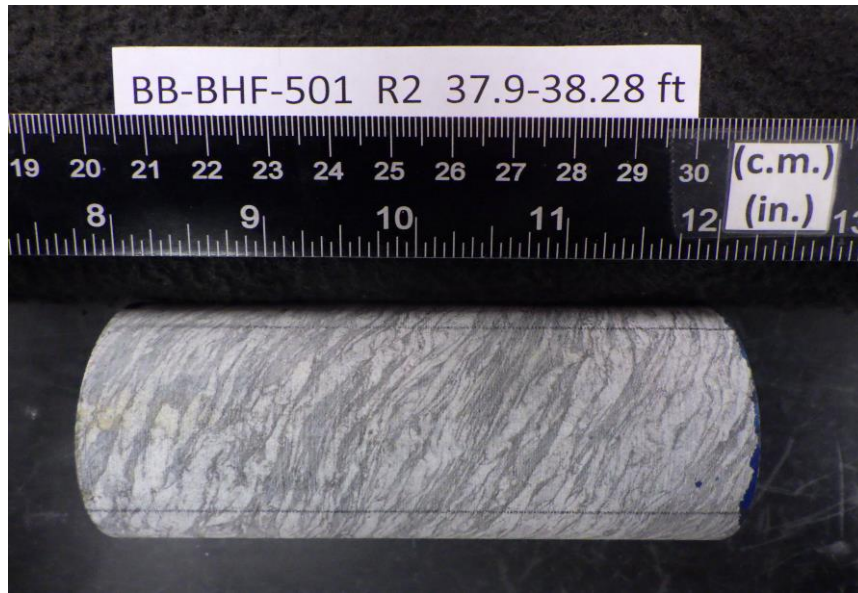
After cutting and grinding
