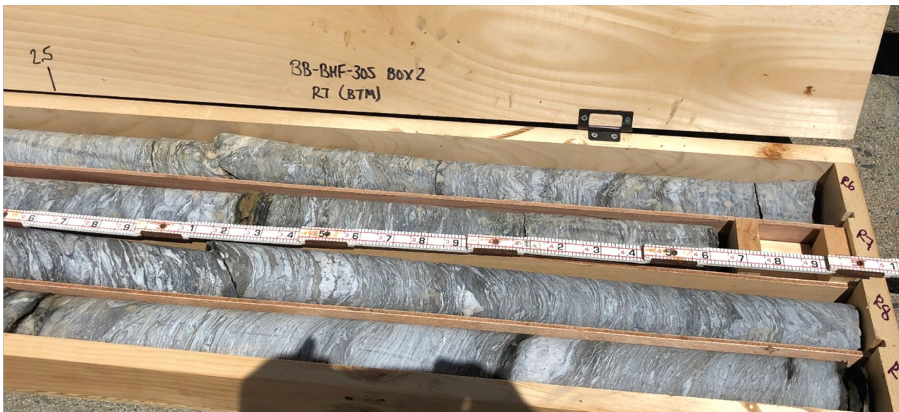
Core box containing dried core from test boring BB-BHF-305 (Box 2 of 2); right side of core box (bottom portion of cores).
