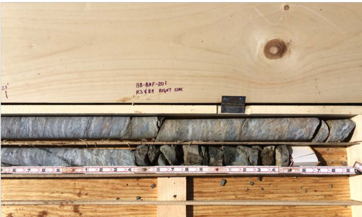
Photo 4: Core box containing dried core from test boring BB-BHF-201: Right side of core box (bottom 2.5-foot portion of cores). Slots from top to bottom: 1) BB-BHF-201, R3 (30 to 35 ft); 2) BB-BHF-201, R4 (35 to 40 ft).
