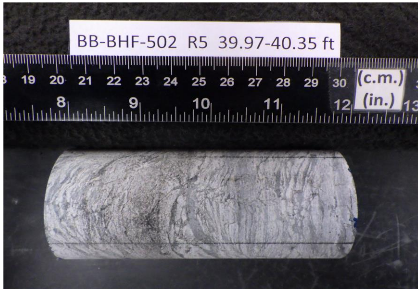
After cutting and grinding
