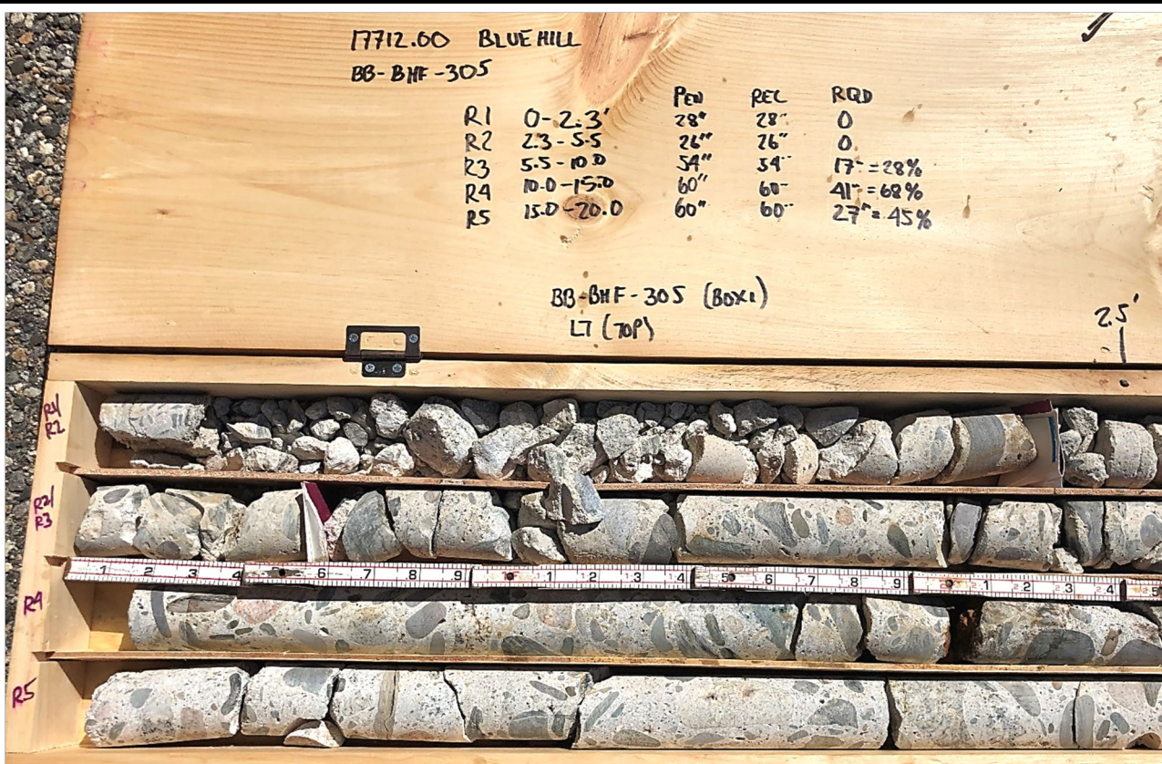
Core box containing dried core from test boring BB-BHF-305 (Box 1 of 2); left side of core box (top portion of cores).
