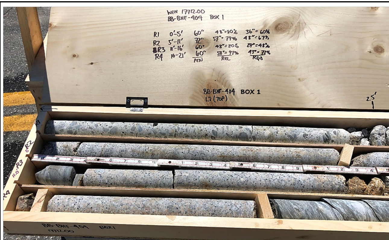
Core box containing dried core from test boring BB-BHF-404 (Box 1 of 2); left side of core box (top portion of cores). Slots from top to bottom:
