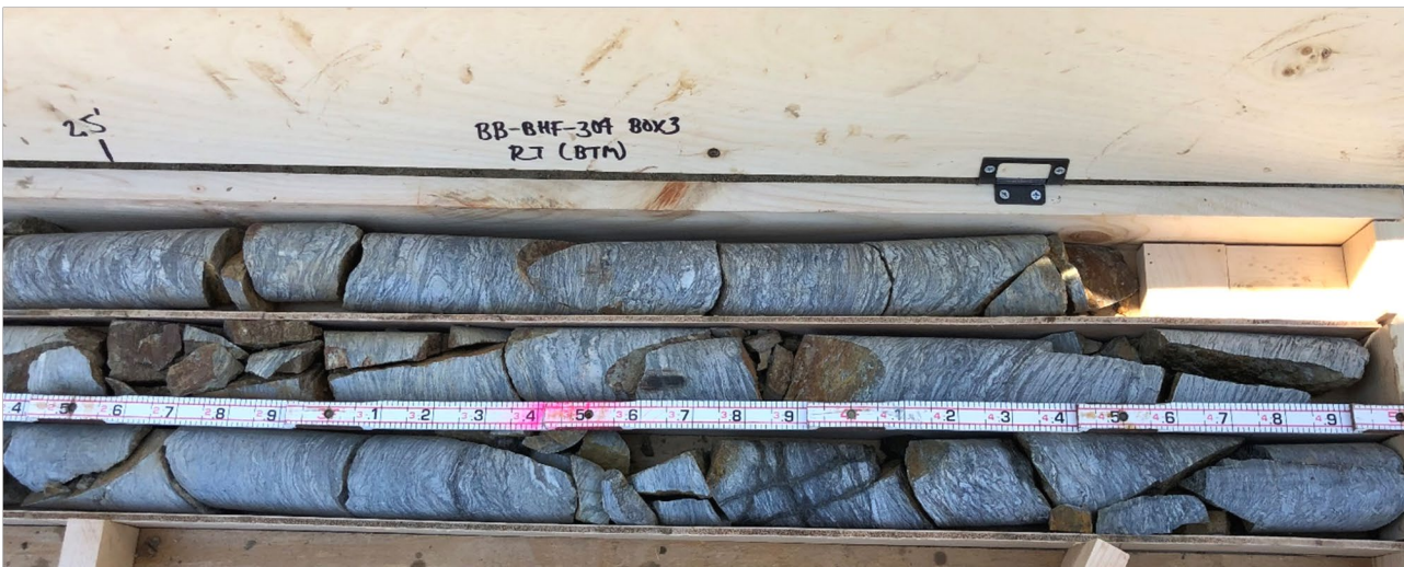
Core box containing dried core from test boring BB-BHF-304 (Box 3 of 3); right side of core box (bottom portion of cores). Slots from top to bottom:
