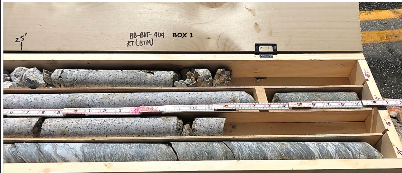
Core box containing dried core from test boring BB-BHF-404 (Box 1 of 2); right side of core box (bottom portion of cores). Slots from top to bottom:
