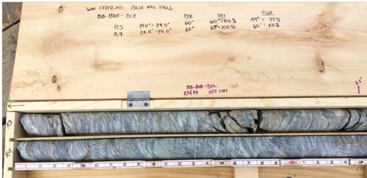
Photo 7: Core box containing dried core from test boring BB-BHF-202: Left side of core box (top 2.5-foot portion of cores).
