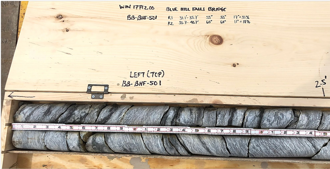
Core box containing dried core from test boring BB-BHF-501 (Box 1 of 1); left side of core box (top portion of cores). Slots from top to bottom:
