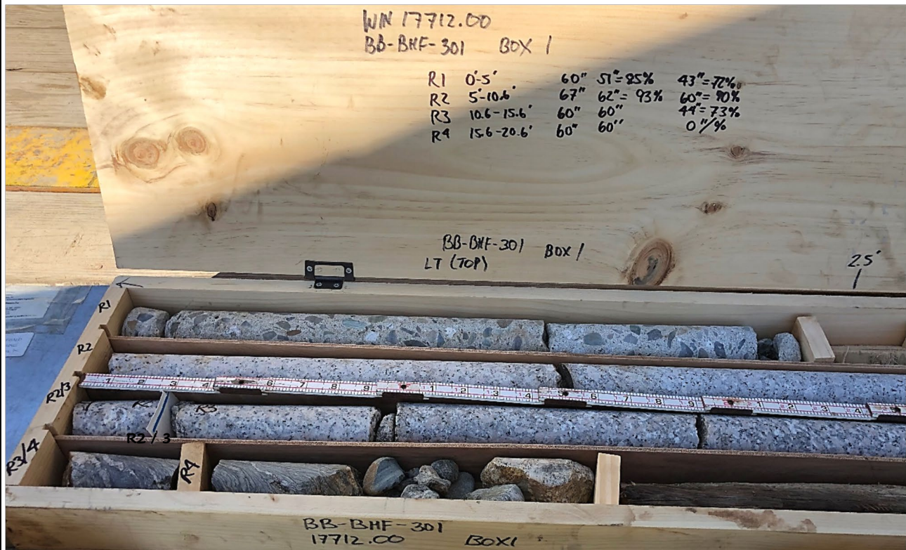
Core box containing dried core from test boring BB-BHF-301 (Box 1 of 1); left side of core box (top portion of cores). Slots from top to bottom:
