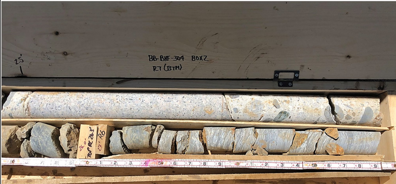
Core box containing dried core from test boring BB-BHF-304 (Box 2 of 3); right side of core box (bottom portion of cores). Slots from top to bottom:
