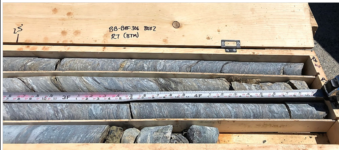
Core box containing dried core from test boring BB-BHF-306 (Box 2 of 2); right side of core box (bottom portion of cores). Slots from top to bottom:
