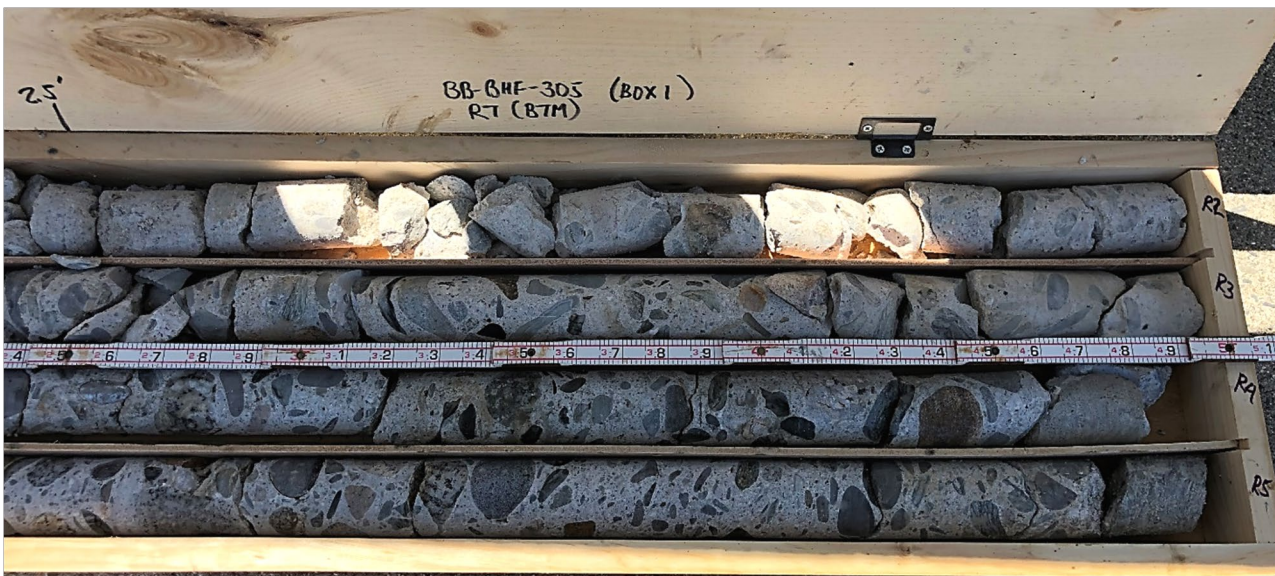
Core box containing dried core from test boring BB-BHF-305 (Box 1 of 2); right side of core box (bottom portion of cores). Slots from top to bottom:
