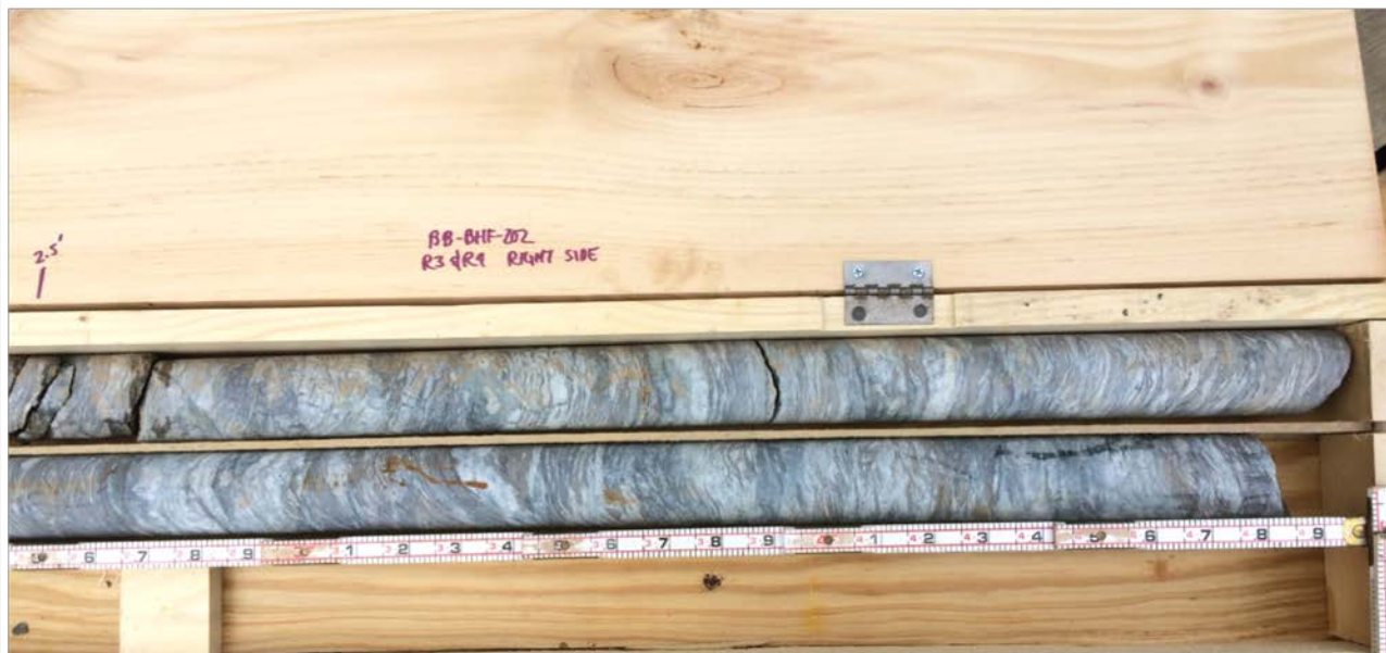
Photo 8: Core box containing dried core from test boring BB-BHF-202: Right side of core box (bottom 2.5-foot portion of cores).
