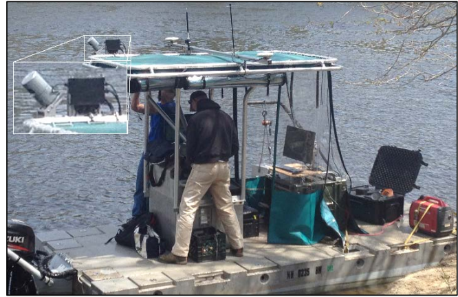
Piper outfitted for combined multibeam and mobile laser scanning operations on a shallow inland river. Laser scanner is mounted on overhead canopy aft of POSMV antennas and multibeam sonar is mounted on port side.
