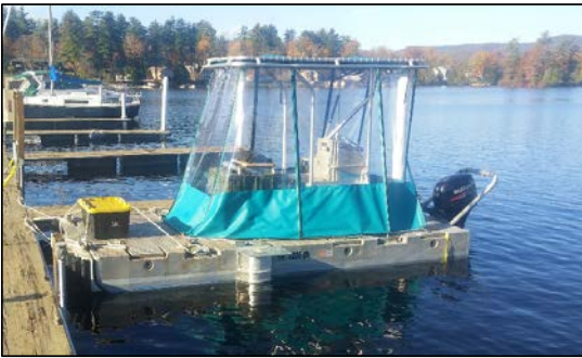
Piper on a large inland lake configured for multibeam survey operations during a period of inclement weather
