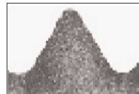
Modified thread: Note stress relieving radii in this unretouched photo enlargement of the supabuckle.
