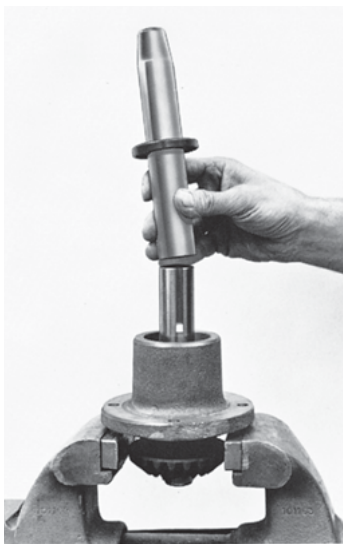
FIGURE 10 – Oil Seal Installation
