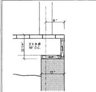
14. BASE @ PORCH DETAIL SCALE: 1 1/2" = 1'-0"
