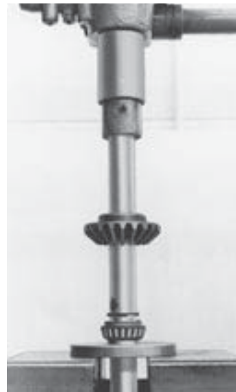
FIGURE 7 – Reassembly of Gear and Bearing Cone
