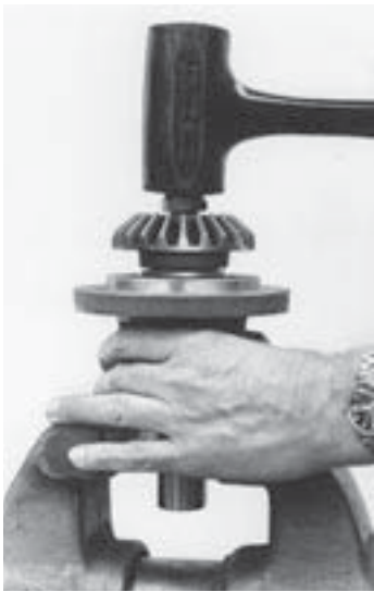
FIGURE 9 – Pinion Assembly Adjustment
