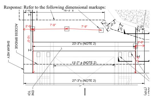
127. Question: Sheet S-181, Rock Anchor Note 5, please confirm that Grade 75 thread bar or hollow bar is acceptable in lieu of Grade 60 deformed bar.
