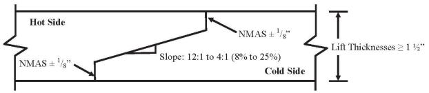
**FIGURE 1: Notched Wedge Joint**
