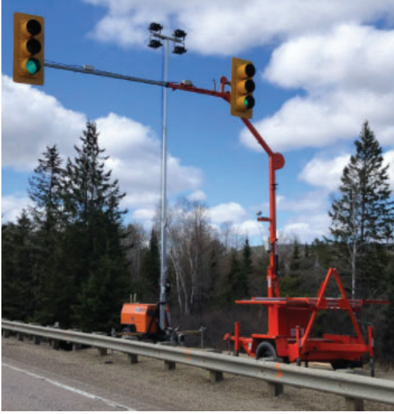
Example of Trailer Mounted type or SQ3
