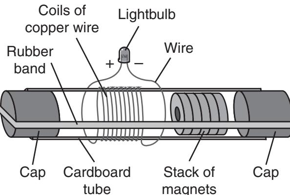
When the students shake the flashlight, the magnets move through the coil of copper wire, and current flows through the wires and bulb.
