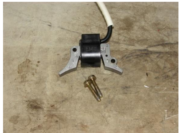
Armature: a part consisting of coils of wire around an iron core that induces an electric current when it is rotated in a magnetic field.
