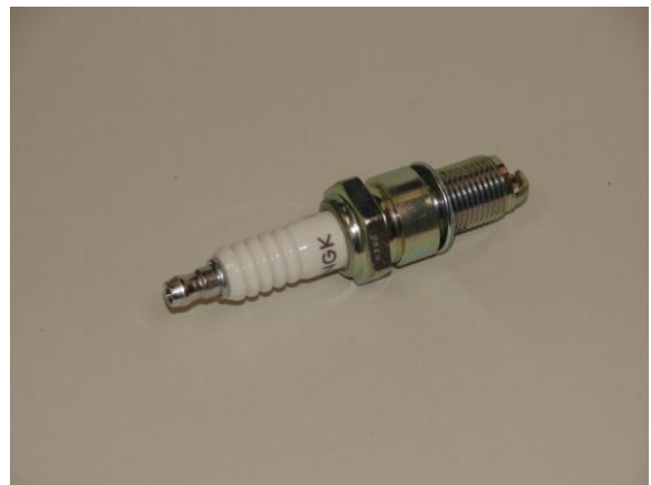
Spark Plug: a device inserted into the combustion chamber of an engine that contains an insulated control electrode for conducting current.
