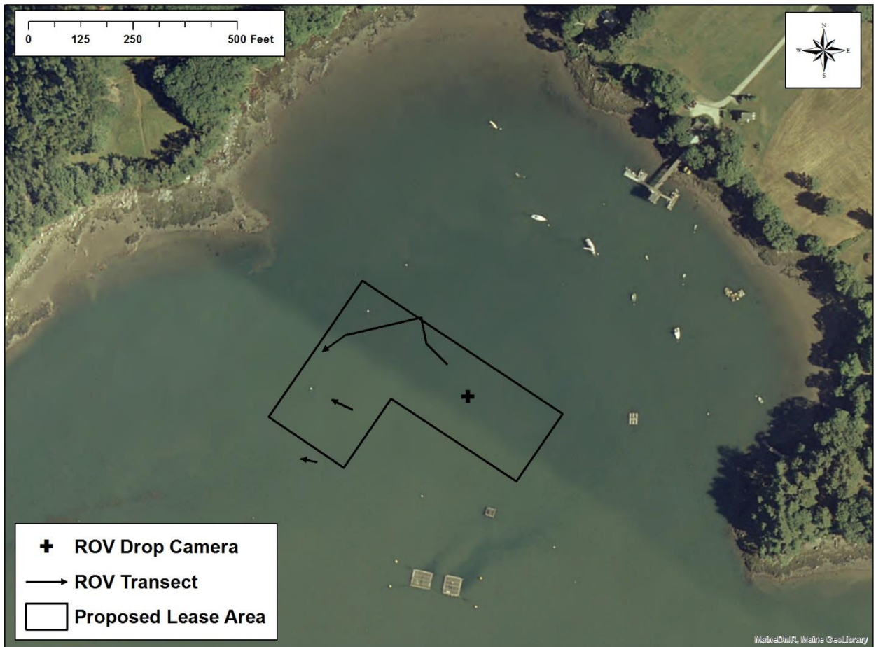
Figure 4. ROV stationary drop and transects conducted on July 6, 2021.
