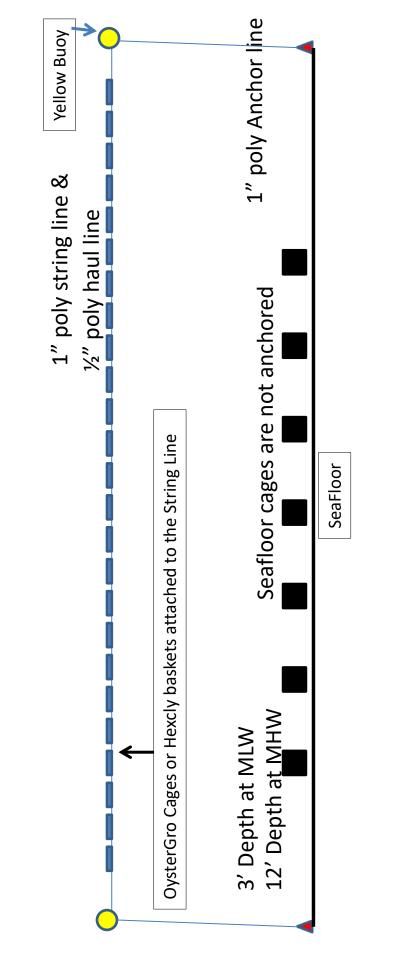
As many as 70 OysterGro Cages on a line over the length of the lease or 600 Hexcyl Baskets. Sinking Cages (36"x45"x32") may be used below or between the string lines.
