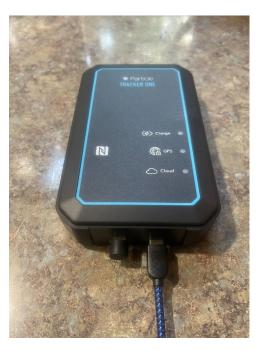
2. Connect the other end of the cable to an available USB A port or to an AC outlet with the provided adapter.
