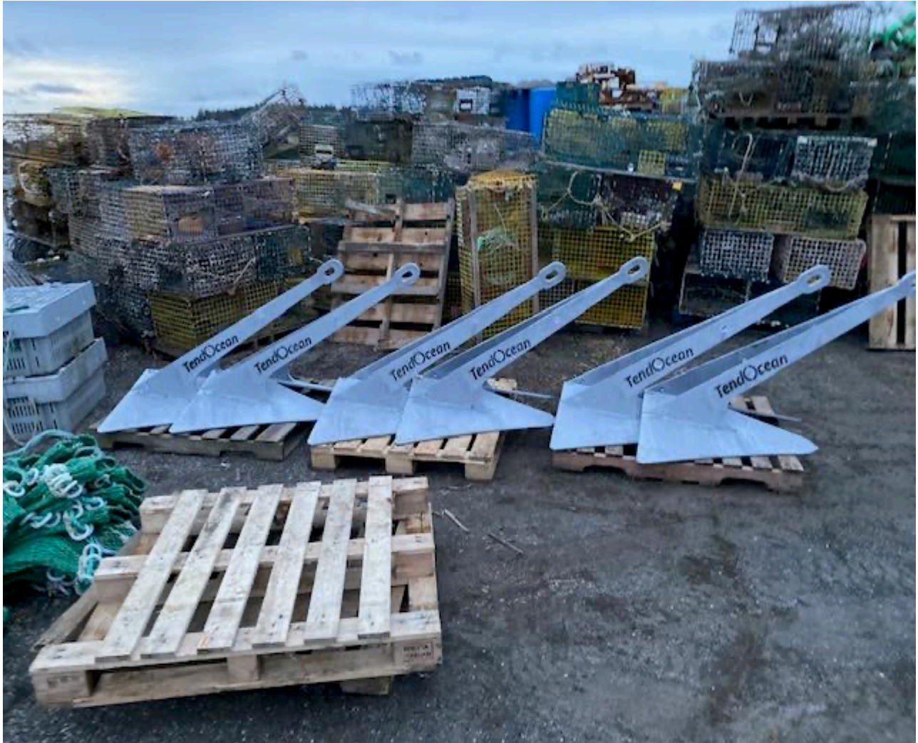
200# TendOcean dual-shank plow anchors
