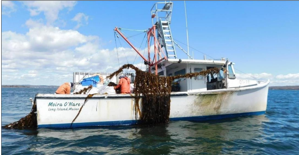
Photo 7. Lobster/fishing vessel, 42ft in length, used for harvesting and transporting of kelp.
