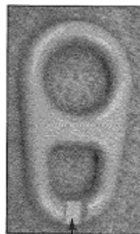
Figure 17. The flat link has a notched section of plastic, which breaks when a force of 600 pounds or greater is applied to it.
