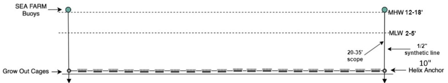
Figure 15: Seasonal Cross Section View of OysterGro Cages for Dodge Cove Marine Farm's proposal.
