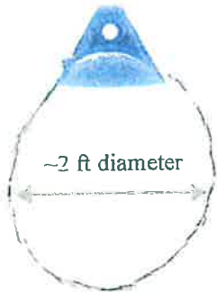
Mooring Ball Description: A3 or A4 Polyballs Height: 23 inches Diameter: ~2 feet
