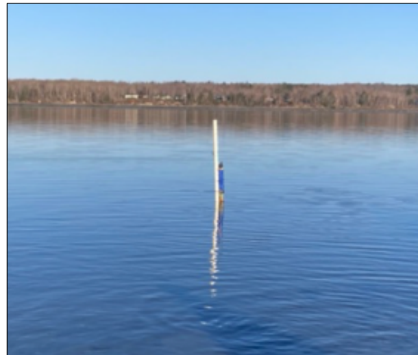
Figure 3. Deployment setup of eelgrass sonde attached to a PVC pole.
