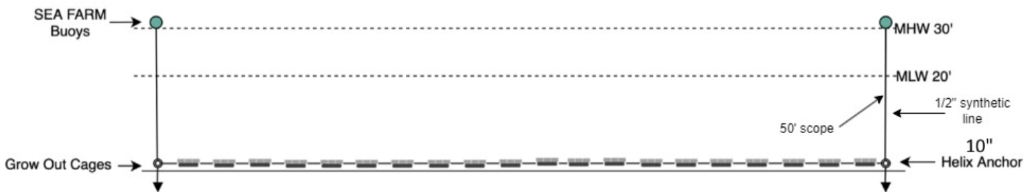
Figure 19: Seasonal Cross Section View for OysterGro Cages in Muscongus Bay Aquaculture's proposal.
