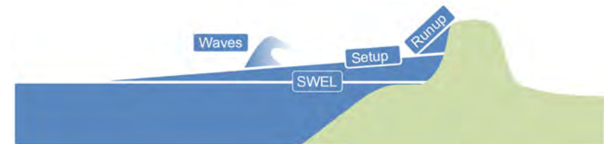
FIGURE 5.2 - Definition sketch of FEMA coastal base flood components. Base flood elevation is a combination of estimated peak storm surge elevation (stillwater elevation [SWEL] plus wave setup) plus wave runup (overland rush of water after waves break). Image reproduced from a FEMA graphic.
