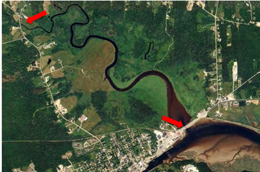
FIGURE 3.1 - Red arrows indicate tidal restrictions in Machias caused by roads in the Middle River, near its outlet and farther upstream. The types of impacts caused by restrictions are strongly tied to their relative position in the system. Image source: Google Earth.
