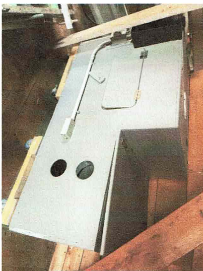
Noise insulated Gen/Pump box 36"x36"x60"
