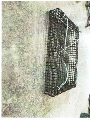
Oyster Grow-out tray 4"x20"x30" (320 trays) 1" vinyl coated wire
