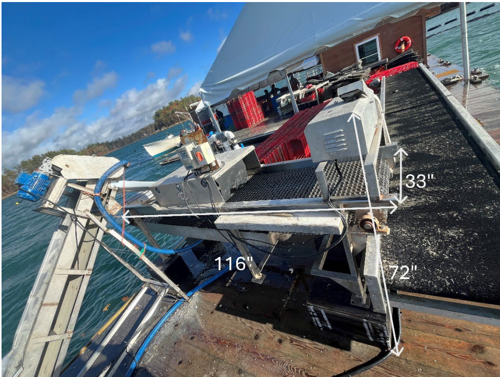
Figure 7: Picture of aluminum wash system for Dodge Cove Marine Farms's proposed amendment. One wash system would be added to the lease.
